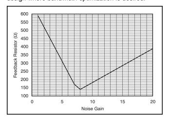
Figure 33. Feedback Resistor vs Noise Gain
