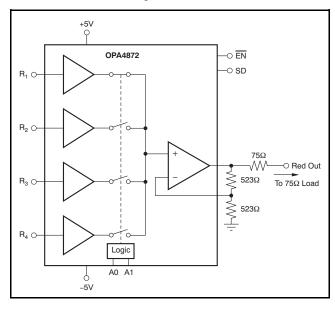
Figure 30. 4-Input RGB Router (Red Channel Shown)
