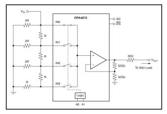
Figure 29. 2-Bit, High-Speed Attenuator, 500MHz Channel Bandwidth
