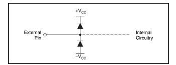
Figure 36. Internal ESD Protection
