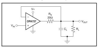
Figure 30. Series Resistor in Unity-Gain Buffer Configuration Improves Capacitive Load Drive
