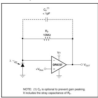
Figure 33. Single-Supply Transimpedance Amplifier
