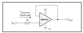
Figure 29. Input Current Protection for Voltages Exceeding the Supply Voltage
