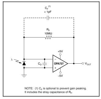
Figure 32. Dual-Supply Transimpedance Amplifier
