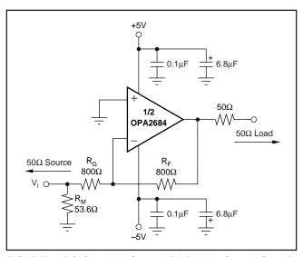
FIGURE 2. DC-Coupled, G = -1V/V, Bipolar Supply Specifications and Test Circuit.
