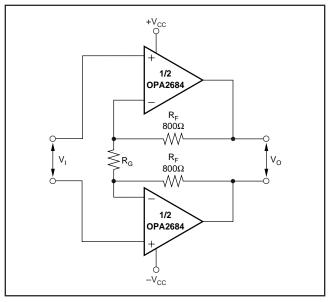
FIGURE 5. Noninverting Differential I/O Amplifier.
