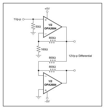
FIGURE 7. Single to Differential Conversion.
