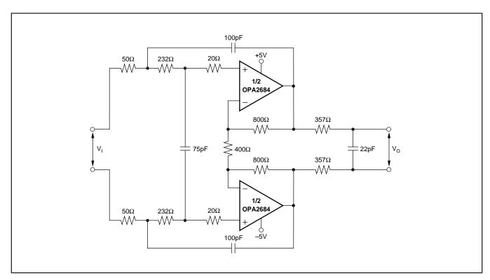
FIGURE 9. Low-Power, Differential I/O, 4th-Order Butterworth Active Filter.
