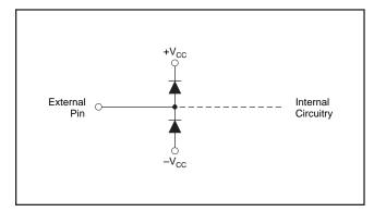
FIGURE 17. Internal ESD Protection.
