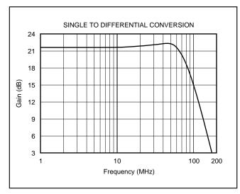
FIGURE 8. Small-Signal Bandwidth for Figure 7.
