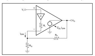
FIGURE 15. Current-Feedback Transfer Function Analysis Circuit.
