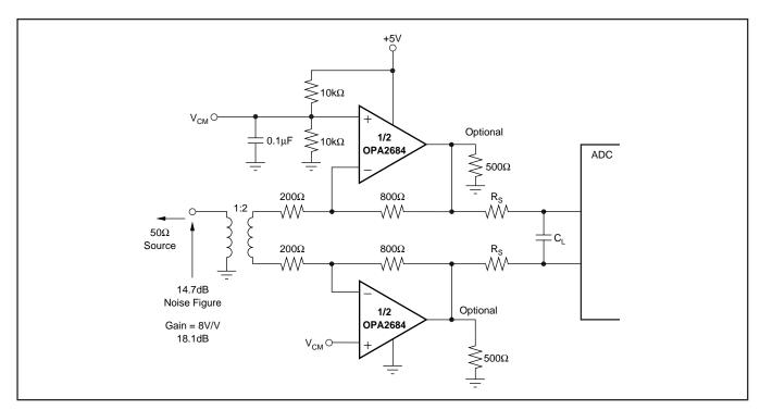
FIGURE 11. Single-Supply Differential ADC Driver.
