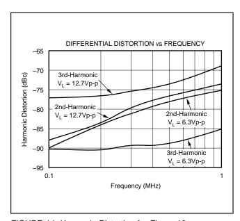
FIGURE 14. Harmonic Distortion for Figure 13.
