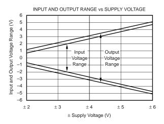
At  $T_A$  = +25°C, G = +2,  $R_F$  = 800 $\Omega$ ,  $R_L$  = 100 $\Omega$ , unless otherwise noted.
