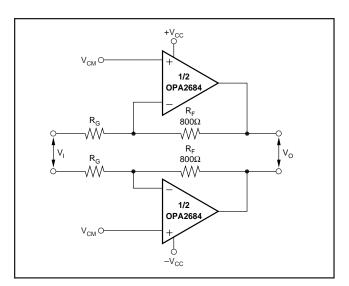
FIGURE 6. Inverting Differential I/O Amplifier.
