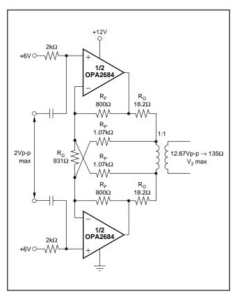
FIGURE 13. Synthetic Output Impedance xDSL Driver.
