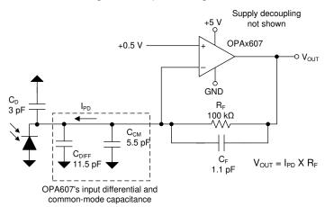
Figure 9-1. Wideband, High-Sensitivity, Transimpedance Amplifier
