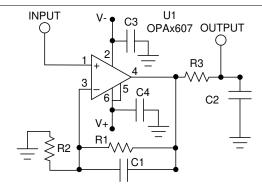
Figure 11-2. Layout Example Schematic
