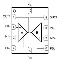
Figure 6-4. OPA2607 RUG Package 10-Pin X2QFN Top View
