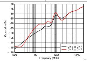
Figure 7-33. Crosstalk vs Frequency
