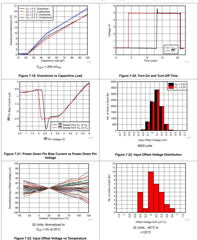
Figure 7-24. Input Offset Drift Distribution
