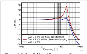
Figure 9-7. Small-Signal Frequency Response in Gains of 3V/V (a) and 6V/V (b)
