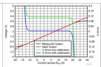
Figure 9-14. DC Current-Sense Transfer Function
