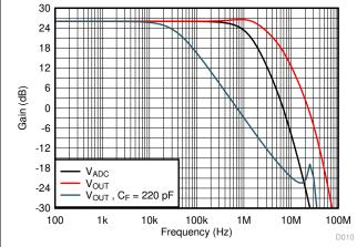
Figure 9-13. Frequency Response of Low Side Current Sensing
