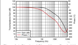
Figure 9-4. Simulated Closed-Loop Bandwidth of TIA
