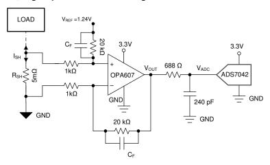
Figure 9-12. Low Side Current Sensing
