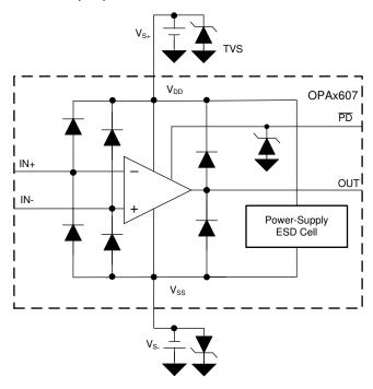
Figure 8-4. Internal ESD Structure
