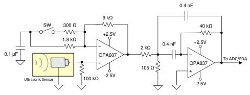
Figure 9-9. Hi-Z, High-Gain Front-End Circuit
