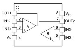
Figure 6-3. OPA2607 D, DGK Package 8-Pin SOIC, VSSOP Top View
