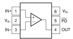
Figure 6-2. DCK Package 6-Pin SC70 **Top View**
