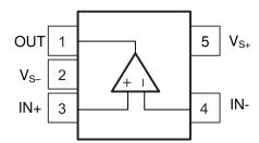
Figure 6-1. DBV Package 5-Pin SOT-23 **Top View**
