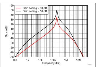
Figure 9-10. Hi-Z, High-Gain Front-End Circuit SNR | Figure 9-11. Hi-Z, High-Gain Front-End Circuit Gain vs Frequency
