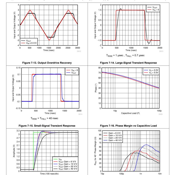
Figure 7-17. Step Settling Time
