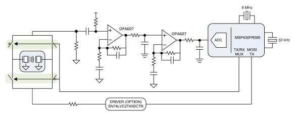
Figure 9-15. High-Gain Ultrasonic Front-End
