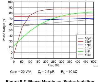
Figure 8-3. Phase Margin vs. Series Isolation Resistor
