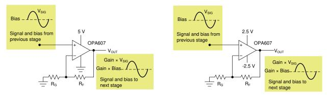
Figure 8-6. Single-Supply and Dual-Supply Operation
