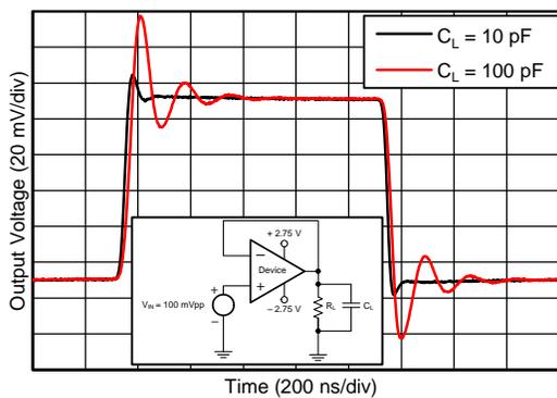
Figure 29. Small-Signal Step Response
