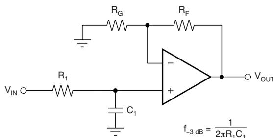
$$\frac{V_{OUT}}{V_{IN}} = \left(1 + \frac{R_F}{R_G}\right) \left(\frac{1}{1 + sR_1C_1}\right)$$
