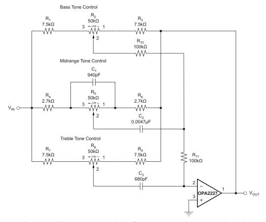
Figure 11. Three-Band ActiveTone Control (Bass, Midrange and Treble)
