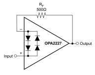
Figure 2. Pulsed Operation
