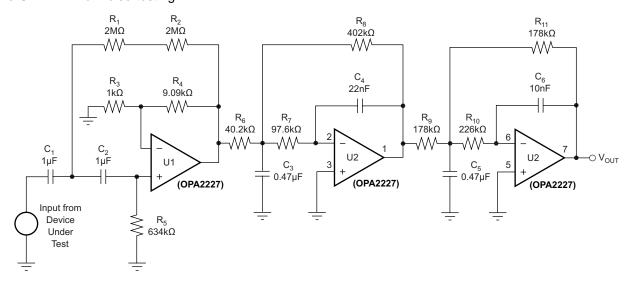
Figure 6. 0.1-Hz to 10-Hz Bandpass Filter Used to Test Wideband Noise of the OPA2227
