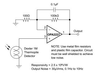
Figure 9. Long-Wavelength Infrared Detector Amplifier
