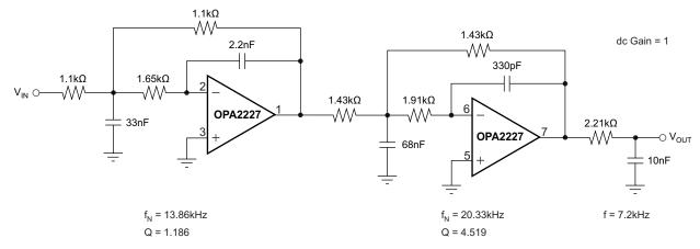
Figure 8. Three-Pole, 20-kHz Low Pass, 0.5-dB Chebyshev Filter
