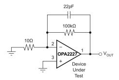
Figure 7. Noise Test Circuit
