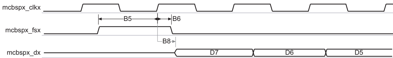
Figure 6-36. McBSP Rising Edge Transmit Timing in Slave Mode
