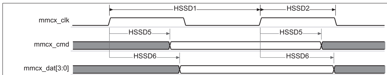
Figure 6-65. MMC/SD/SDIO – High-Speed SD Mode – Data/Command Receive
