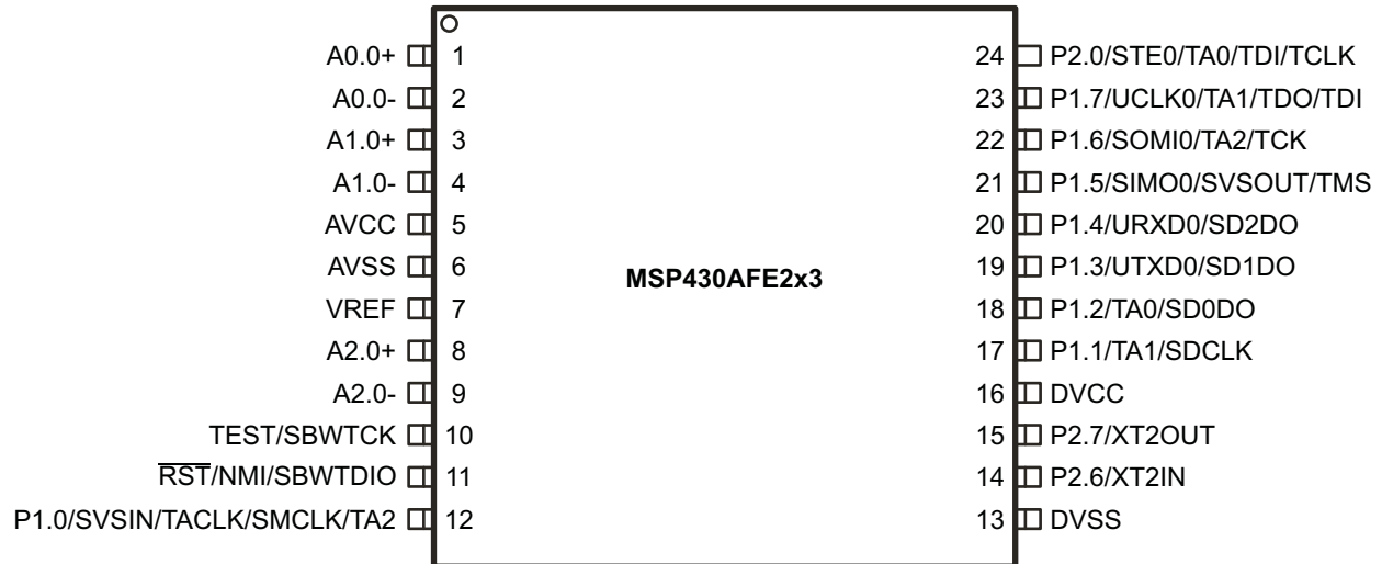
Figure 4-1. 24-Pin PW Package (Top View), MSP430AFE2x3
