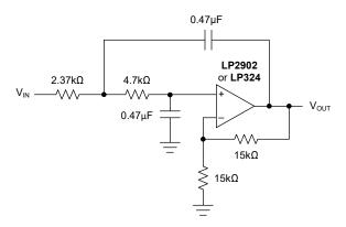
100Hz Low-Pass Filter With a Gain of 2
