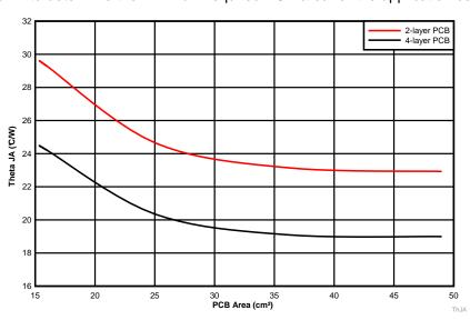
Figure 42.  $\theta_{JA}$  vs PCB Area
