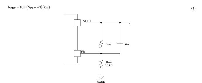
Figure 18. Setting the Output Voltage
