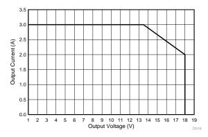
Figure 19. Output Current vs Output Voltage
