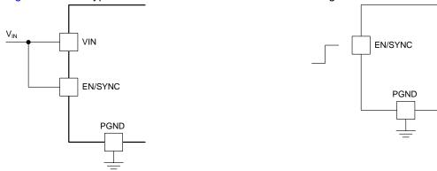
Figure 27. Enabling the Device
