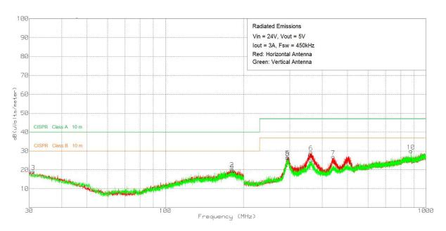
Figure 43. Radiated Emissions 24-V Input, 5-V Output, 3-A Load (EN55011 Class B)
