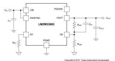
Figure 35. LMZM33603 Typical Schematic
