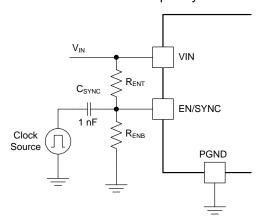
Figure 26. AC-Coupled SYNC Signal
