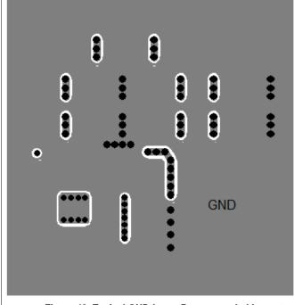
Figure 48. Typical GND-Layer Recommended Layout
