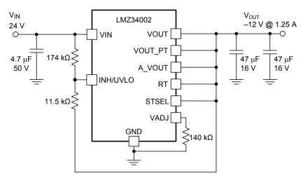
Figure 34. Typical Schematic  $V_{IN} = 24 \text{ V}, V_{OUT} = -12 \text{ V}$
