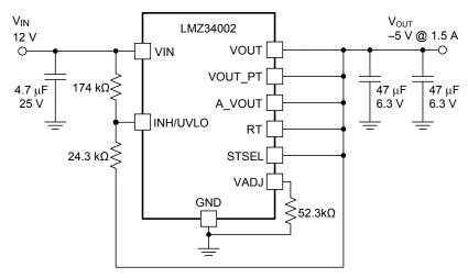
Figure 35. Typical Schematic  $V_{IN} = 12 \text{ V}, V_{OUT} = -5 \text{ V}$
