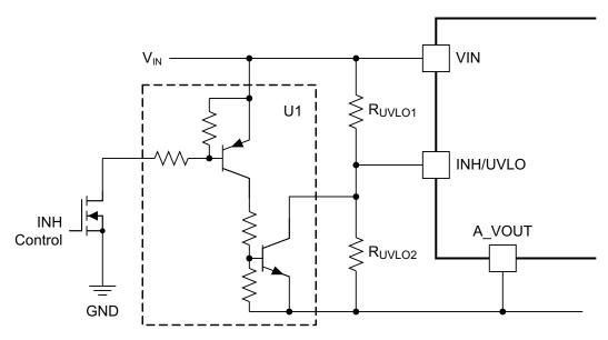
Figure 42. Typical Inhibit Control
