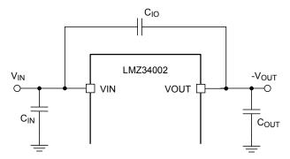
Figure 46. Input to Output Coupling Capacitor
