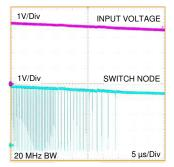
Figure 7-3. High Duty Cycle Operation and Switching Frequency Reduction
