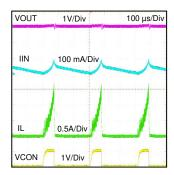
Figure 7-2. Hiccup Behavior with Persistent Output Short Circuit.
