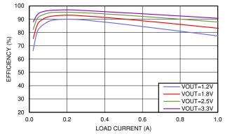
Typical Efficiency at V<sub>IN</sub> = 3.6 V
