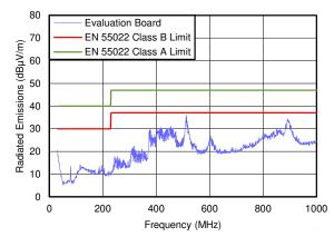
Radiated EMI (CISPR22)  $V_{IN} = 5 \text{ V}$ ,  $V_{OUT} = 1.8 \text{ V}$ ,  $I_{OUT}$ = 1 A
