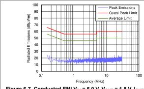
Figure 6-7. Conducted EMI  $V_{IN}$  = 5.0 V,  $V_{OUT}$  = 1.8 V,  $I_{OUT}$  = 1-A Default Evaluation Board BOM with Additional 2.2- $\mu$ h 1- $\mu$ f LC Input Filter
