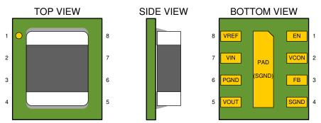
Figure 5-1. SIL Package, 8-Pin µSIP
