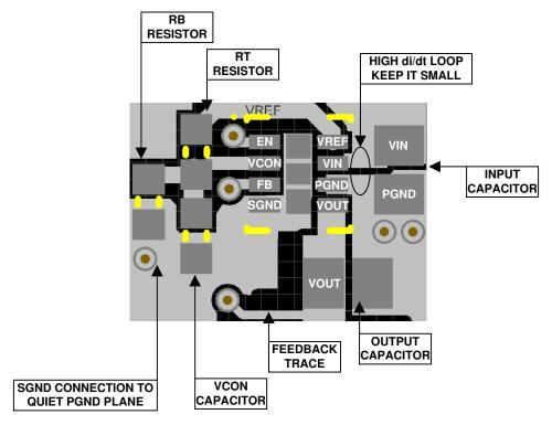
Figure 8-26. Example Top Layer Board Layout
