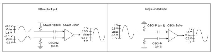
Figure 7-1. Differential vs. Single-Ended Mode
