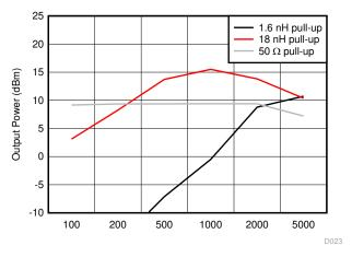
Figure 8-7. Output Power vs Pullup Type
