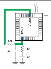
Figure 8-10. External Loop Filter
