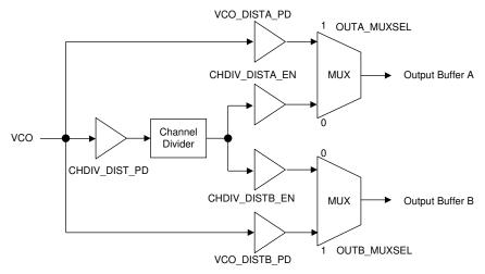
Figure 7-3. Output Distribution Diagram
