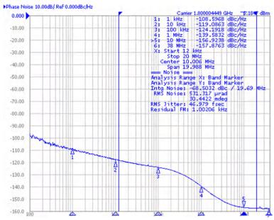
Figure 8-12. Typical Jitter
