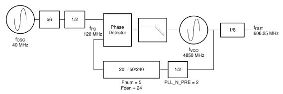
Figure 8-1. Spur Offset Frequency Example
