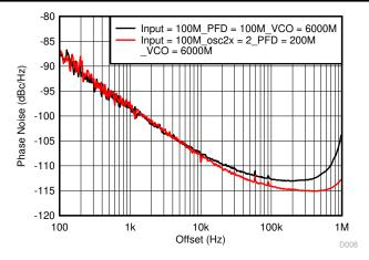
Figure 8-4. 100-MHz Input With OSCin Doubler
