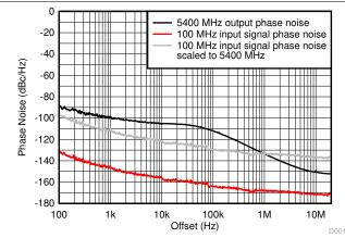
Figure 8-2. Phase Noise of 5.4-GHz Output With Low-Noise Input Signal
