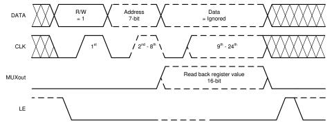
Figure 7-4. Register Readback Timing Diagram
