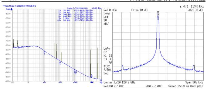
Figure 8-6. Moving Away From Fvco % Fpd Spur
