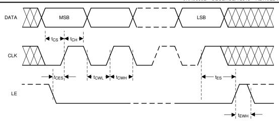
Figure 6-1. Serial Data Input Timing Diagram
