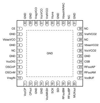
Figure 5-1. RHA Package 40-Pin VQFN Top View
