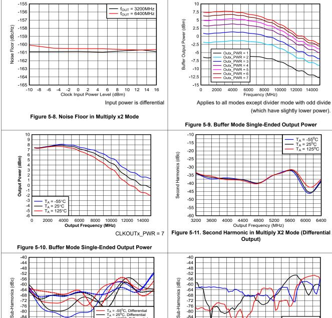
Output Frequency (MHz) Figure 5-12. Multiplier 1/2 Sub-Harmonic in X2 Mode
