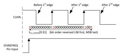
Figure 6-10. SYSREF Windowing to Select the Edge Position for SYNC
