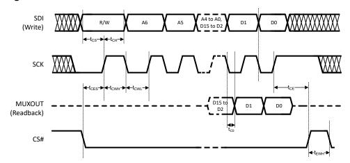
Figure 5-1. Serial Data Input Timing Diagram
