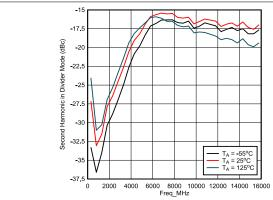
Figure 5-14. Second Harmonic on Divider Mode (Single-Ended Input)
