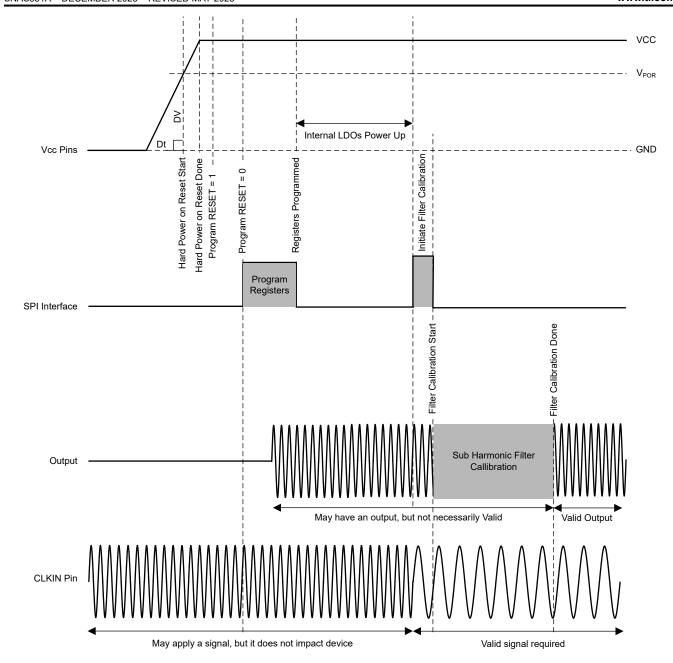
Figure 8-10. Power-Up Timing
