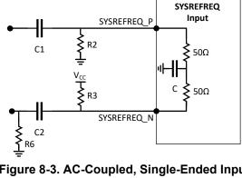
Figure 8-3. AC-Coupled, Single-Ended Input
