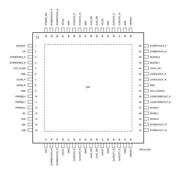
Figure 4-1. PAP0064E Package 64-Pin HTQFP Top View
