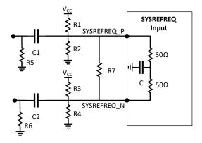
Figure 8-1. SYSREFREQ Input Circuit Recommendations
