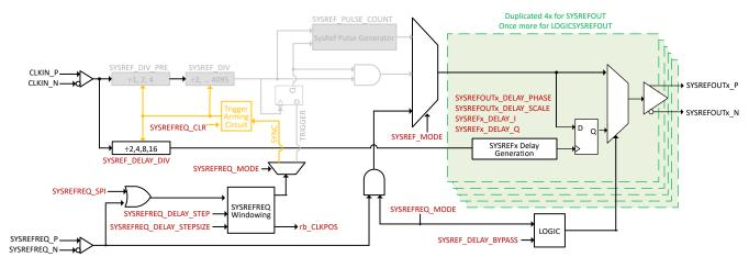
Figure 6-5. Functional Block Diagram of SYSREF Circuitry in Repeater Mode
