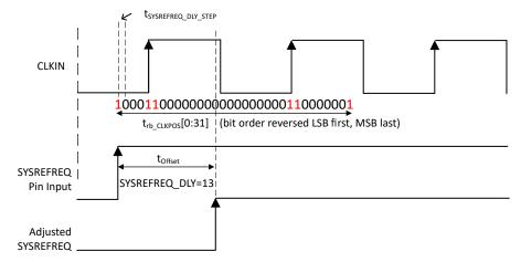
Figure 6-8. SYSREFREQ Internal Timing Adjustment
