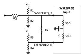
Figure 8-5. DC-Coupled, Single-Ended Input
