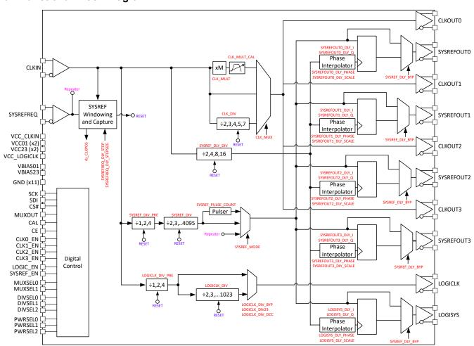
Figure 6-1. Functional Block Diagram
