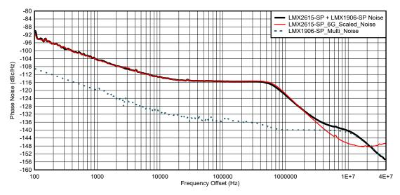
Figure 8-8. LMX1906-SP Multiplier Output
