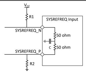
Figure 6-6. SYSREFREQ Pin Logic Low Setup
