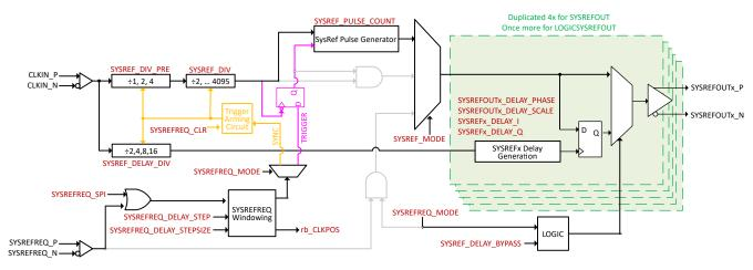
Figure 6-4. Functional Block Diagram of SYSREF Circuitry in Pulser Mode
