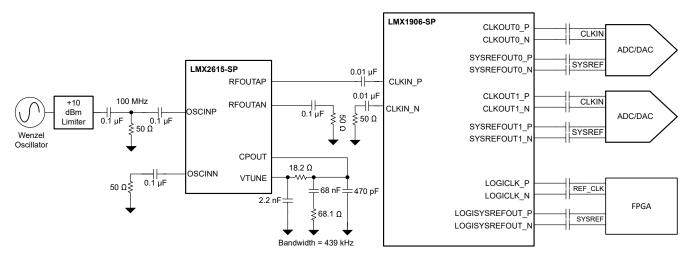
Figure 8-9. Typical JESD Clocks Block Diagram
