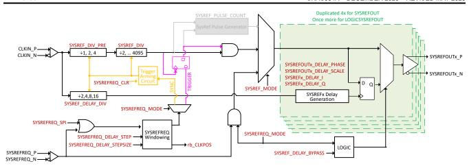
Figure 6-3. Functional Block Diagram of SYSREF Circuitry in Generator Mode
