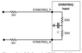
Figure 8-4. DC-Coupled Differential Input
