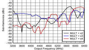
Figure 5-13. Multiplier Sub-Harmonics (Harmonic Frequency = Output Frequency / M )
