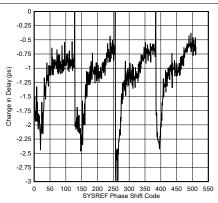
Figure 5-16. SYSREF Delta Delay vs. Code
