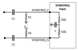
Figure 8-2. AC-Coupled Differential Input
