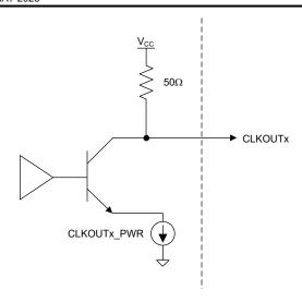
Figure 6-2. CLKOUT Output Buffer
