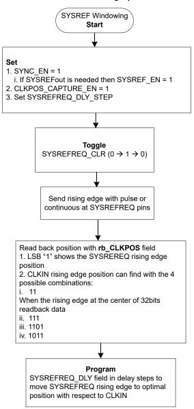
Figure 6-9. Flowchart for SYSREF Windowing Operation
