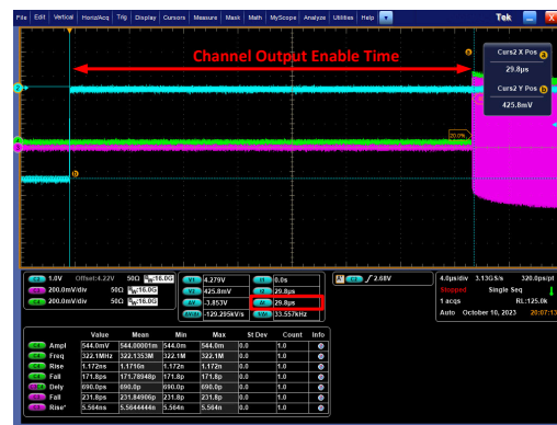
Figure 5-19. Channel Enable Setting Time
