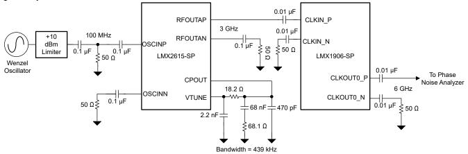
Figure 8-6. Typical Application Schematic
