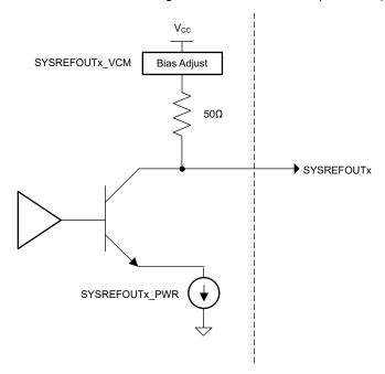
Figure 6-7. SYSREF Output Buffer
