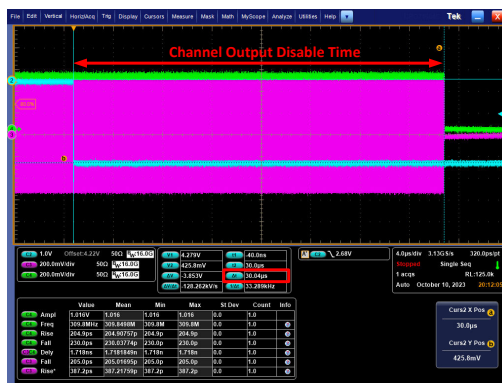
Figure 5-20. Channel Disable Setting Time
