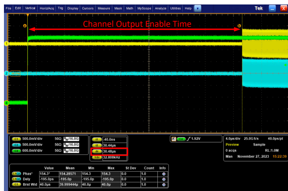
Figure 5-14. Channel Enable Setting Time
