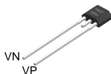
LPG Package 2-Pin TO-92 Top View
