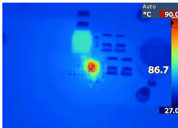
LMR66430MC3 V_{OUT} = 3.3\text{ V} 12 V_{IN} , 3 A, 2.2 MHz Fixed
