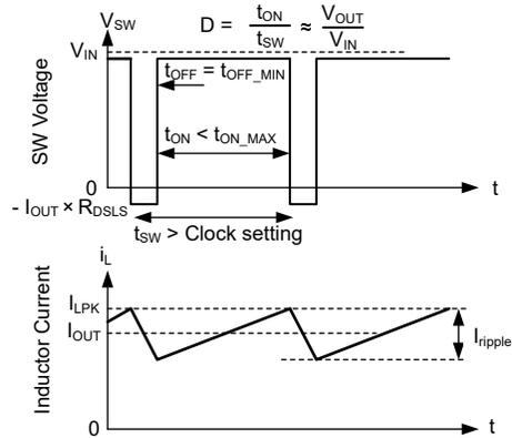
**Figure 7-11. Dropout Waveforms**
