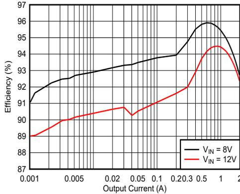
$V_{OUT} = 5V$   $F_{SW} = 400kHz$  Mode = Auto
