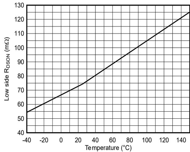
Figure 6-4. Low side MOSFET R\_DS-ON
