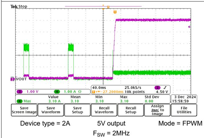
Figure 8-22. Short-Circuit Recovery
