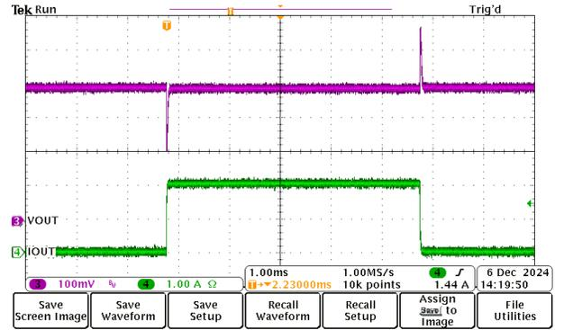
Device type = 2A      5V output      Mode = FPWM
