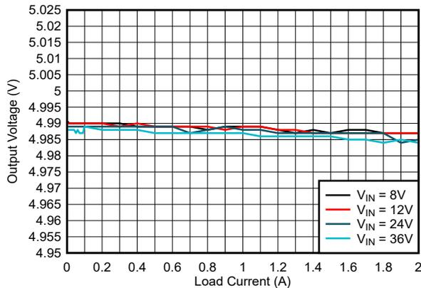
Device type = 2A 5V output Mode = FPWM
