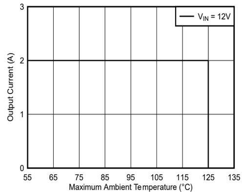
$V_{OUT} = 5V$   $F_{SW} = 400kHz$   $I_{OUT} = 2A$
