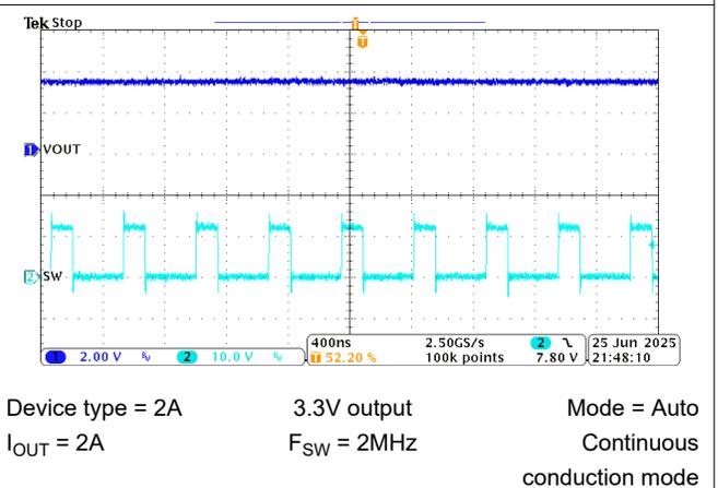
Figure 8-23. Steady State Waveform
