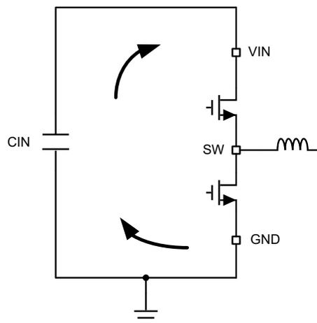
**Figure 8-36. Current Loops With Fast Edges**
