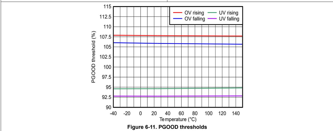
Figure 6-11. PGOOD thresholds
