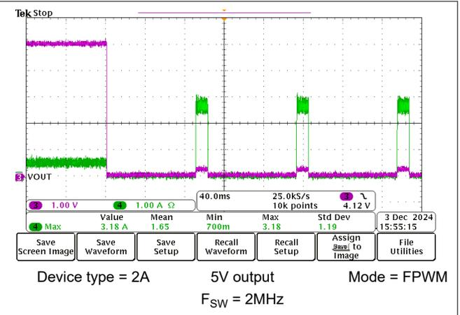
Figure 8-21. Short-Circuit Applied
