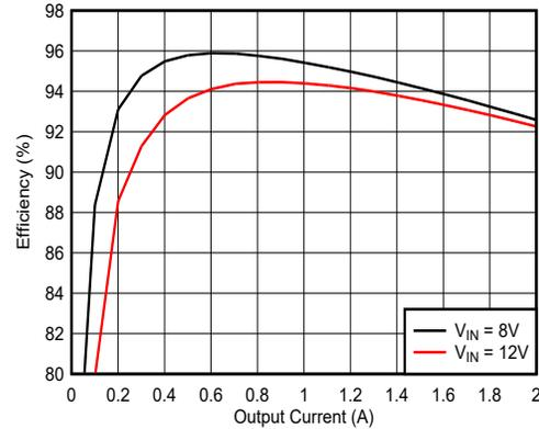
$V_{OUT} = 5V$   $F_{SW} = 400kHz$  Mode = FPWM
