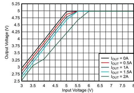
Device type = 2A 5V output Mode = FPWM
