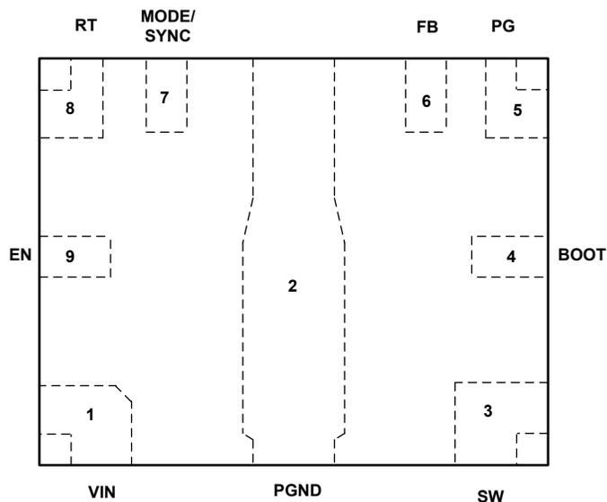
**Figure 5-1. RAK Package 9-Pin WQFN-HR
