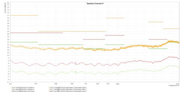
$V_{OUT} = 3.3\text{V}$        $F_{SW} = 2\text{MHz}$        $I_{OUT} = 4\text{A}$
