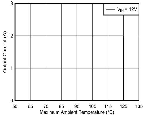
$V_{OUT} = 5V$        $F_{SW} = 2MHz$        $I_{OUT} = 2A$
