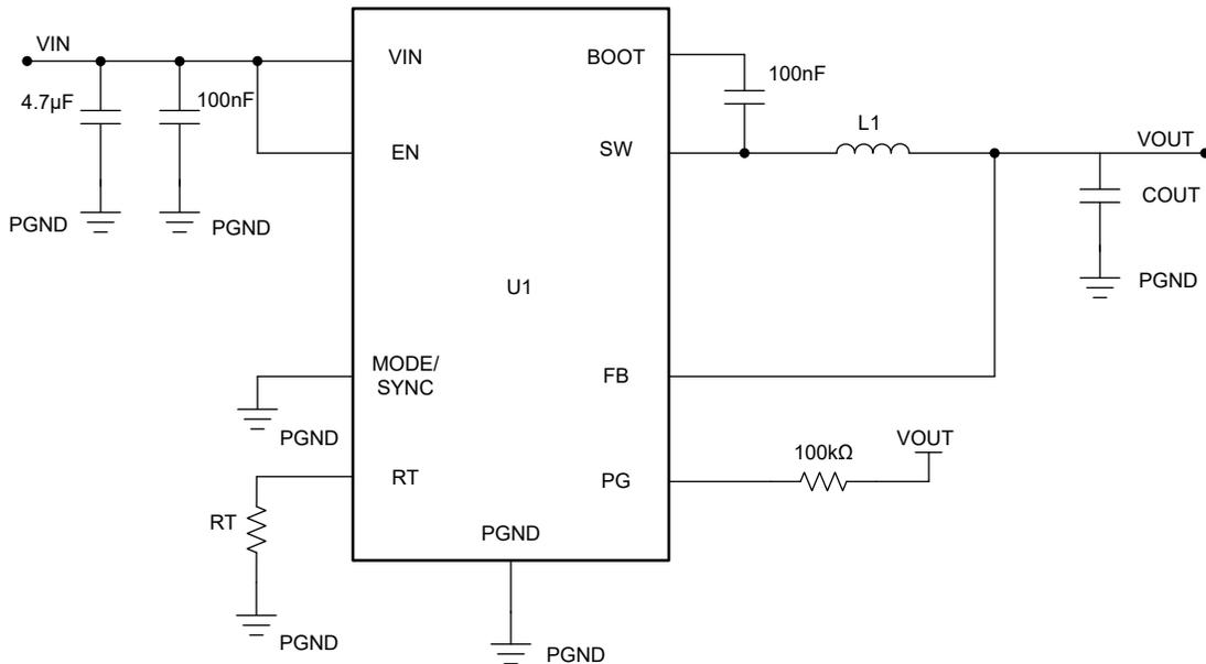
**Figure 8-35. Example Application Circuit**
