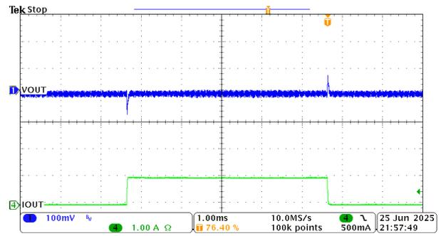
Device type = 2A      3.3V output      Mode = FPWM
