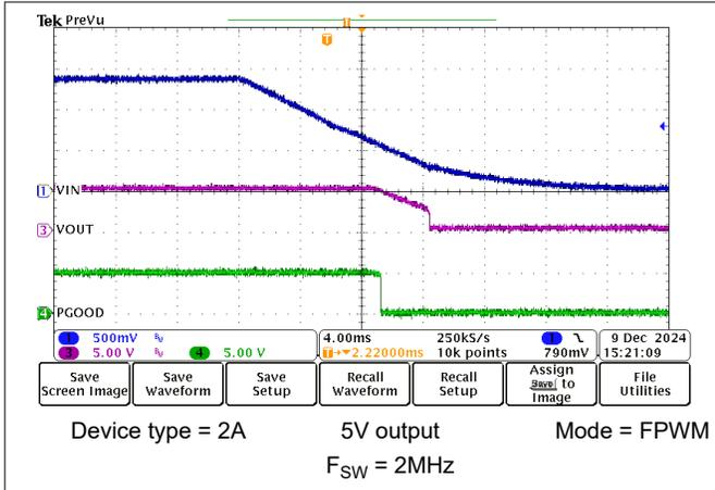
Figure 8-20. Shutdown Operation
