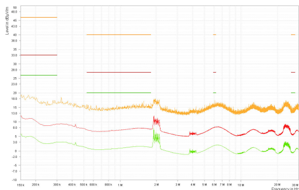
Figure 8-26. Conducted EMI versus CISPR25 Limits (Purple: Peak Signal, Green: Average Signal), LMR60410QEV
