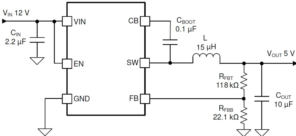
**Figure 8-1. Application Circuit**
