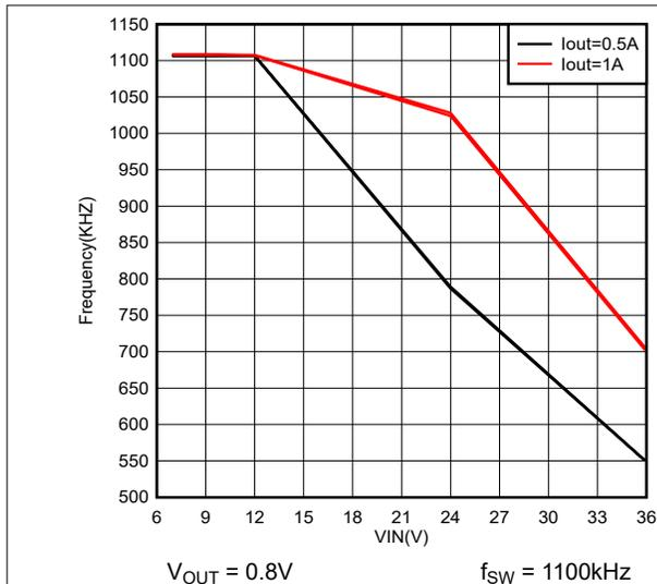
Figure 7-4. Frequency Foldback at T<sub>ON\_MIN</sub>
