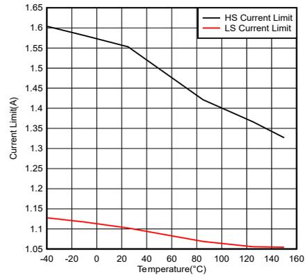
**Figure 6-14. HS and LS Current Limit Versus Temperature-
