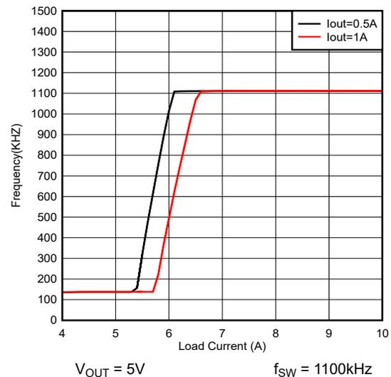
Figure 7-5. Frequency Foldback at T<sub>OFF\_MIN</sub>
