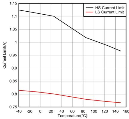
**Figure 6-13. HS and LS Current Limit Versus Temperature-
