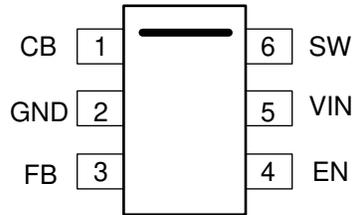
**Figure 5-1. 6-Pin SOT-23 DBV Package (Top View)**
