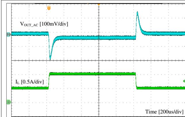
Figure 8-7. Load Transient
