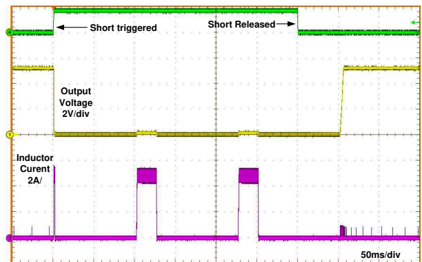
Figure 8-6. Short-Circuit Transient and Recovery
