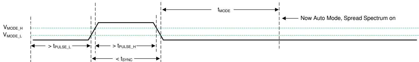
Figure 8-10. Transition from SYNC Mode to Auto Mode
