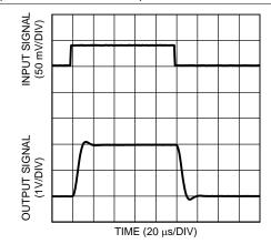
Figure 19. Step Response at V  $_{S}$  = 3.3 V, R  $_{L}$  = 10 k  $\Omega$  LMP8602 and LMP8602-Q1
