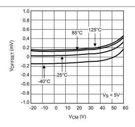
Figure 2.  $V_{OS}$  vs  $V_{CM}$  at  $V_S = 5$  V
