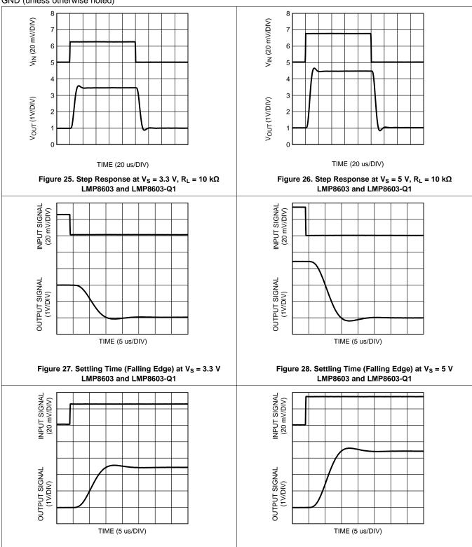
Figure 29. Settling Time (Rising Edge) at V<sub>S</sub> = 3.3 V
