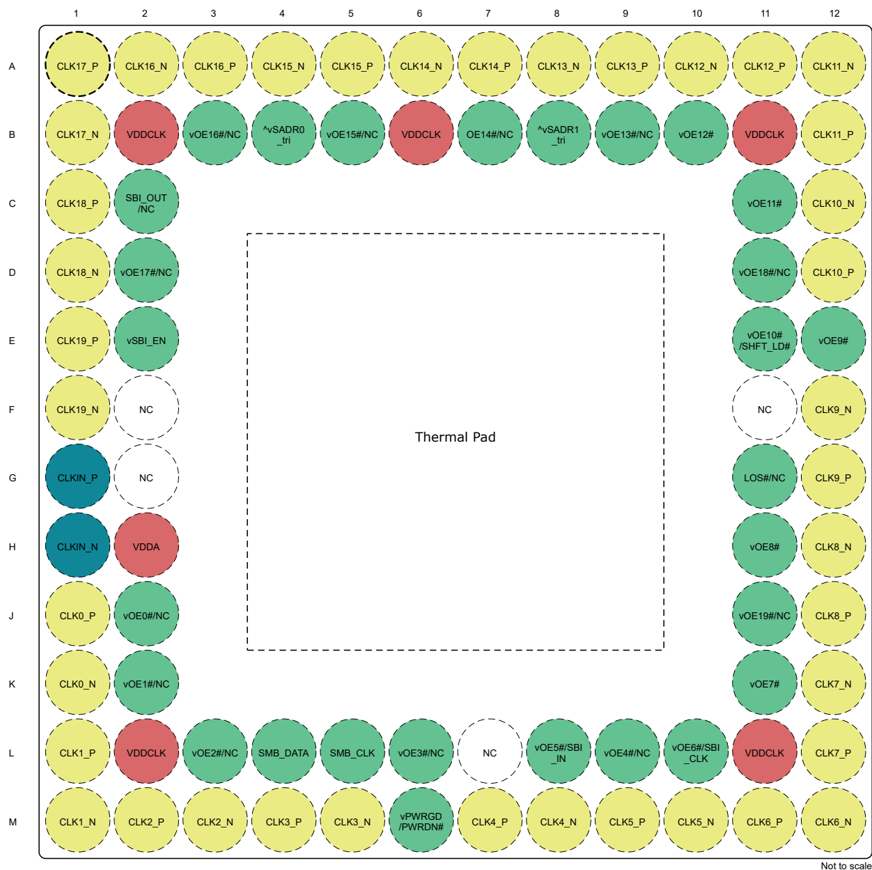
Figure 5-1. LMKDB1120 and LMKDB1120FS 6mm x 6mm NPP Package 80 Pin TLGA Top View
