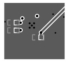
Figure 9-9. PCB Layout Example for LMK3H0102, Bottom Layer
