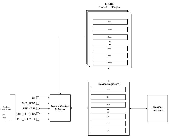
Figure 7-3. LMK3H0102 Interface and Control Blocks
