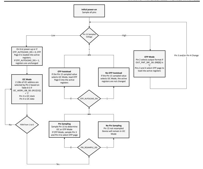
Figure 7-2. LMK3H0102 Device Mode Diagram
