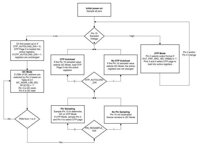
Figure 7-2. LMK3H0102 Device Mode Diagram
