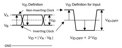
Figure 6-7. Two Different Definitions for Differential Input Signals
