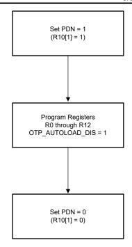
Figure 7-4. LMK3H0102 Programming Sequence
