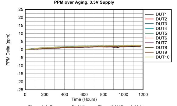
Figure 9-9. Frequency Stability over Time - 3.3V Supply Voltage
