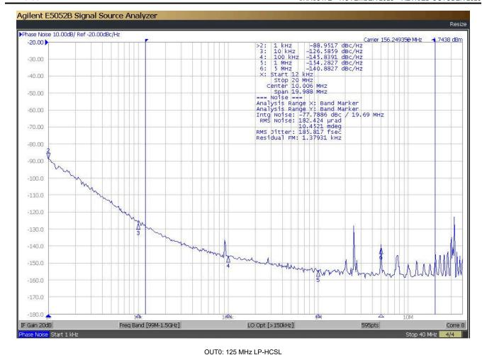
OUT1: 156.25 MHz LP-HCSL Temperature: 25 °C 12k – 20M RMS Jitter: 186 fs
