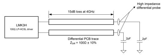
Figure 6-5. LP-HCSL Output Configuration During PCle Device Test
