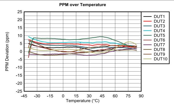
Figure 9-10. Frequency Stability over Temperature
