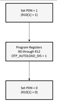
Figure 7-4. LMK3H0102 Programming Sequence
