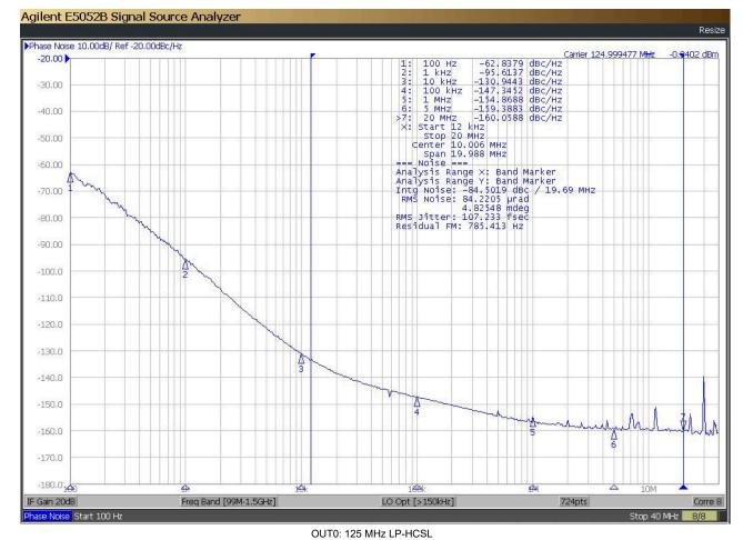
OUT1: 125 MHz LP-HCSL Temperature: 25 °C 12k – 20M RMS Jitter: 107 fs
