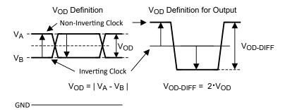
Figure 6-8. Two Different Definitions for Differential Output Signals
