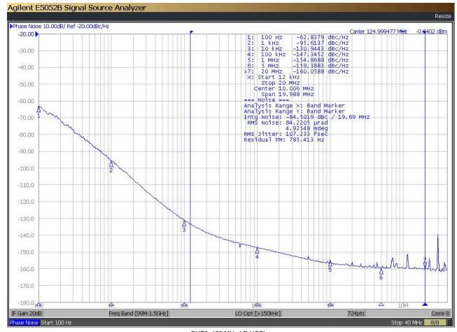
OUT0: 125 MHz LP-HCSL OUT1: 125 MHz LP-HCSL Temperature: 25 °C 12k – 20M RMS Jitter: 107 fs
