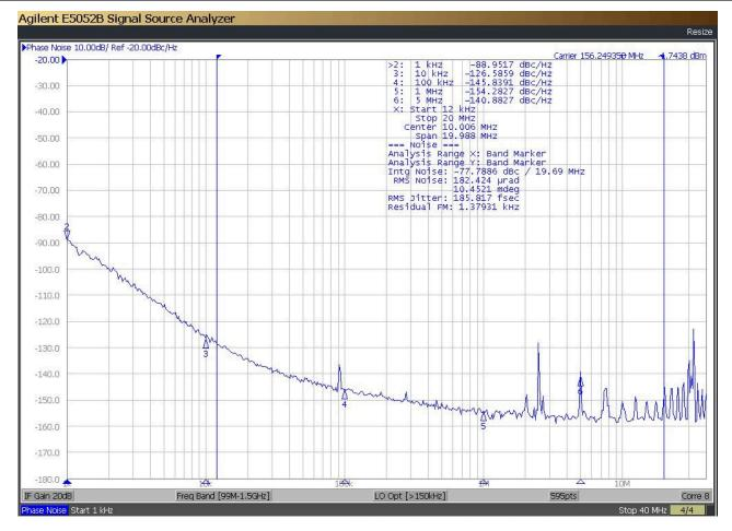
OUT0: 125 MHz LP-HCSL OUT1: 156.25 MHz LP-HCSL Temperature: 25 °C 12k – 20M RMS Jitter: 186 fs
