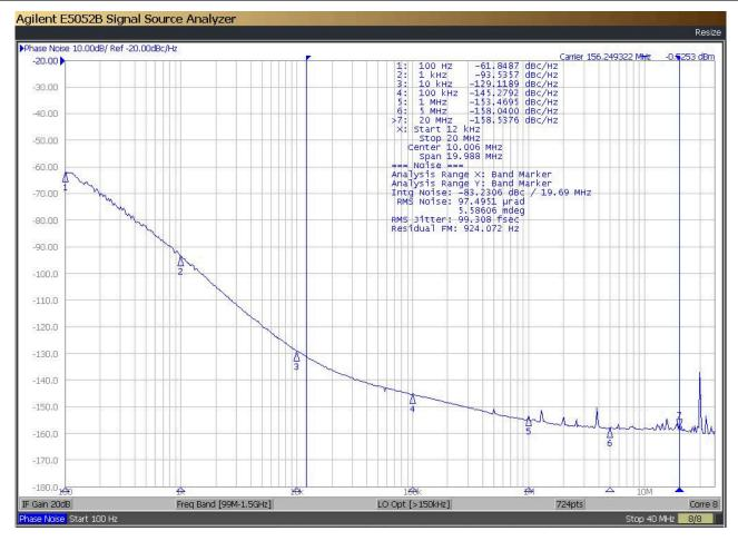
OUT0: 156.25 MHz LP-HCSL OUT1: 156.25 MHz LP-HCSL Temperature: 25 °C 12k – 20M RMS Jitter: 99 fs
