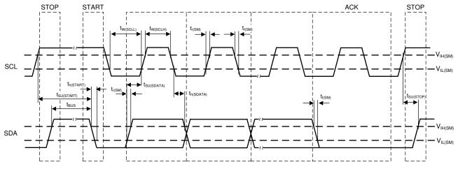
Figure 7-9. I<sup>2</sup>C Timing Diagram
