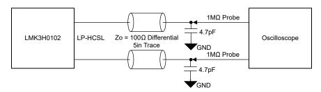
Figure 6-4. LP-HCSL Output Configuration During Non-PCIe Device Test
