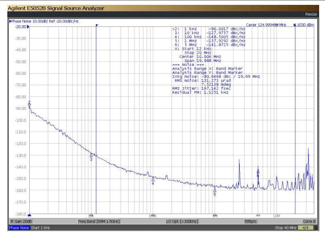
OUT0: 125 MHz LP-HCSL OUT1: 156.25 MHz LP-HCSL Temperature: 25 °C 12k – 20M RMS Jitter: 167 fs
