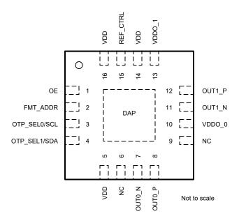
Figure 4-1. LMK3H0102 16-Pin TQFN Top View
