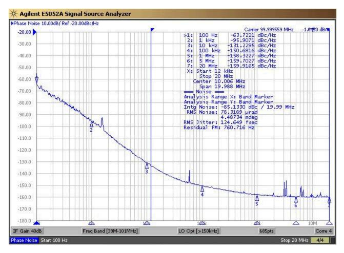
OUT0: 100 MHz LP-HCSL OUT1: 100 MHz LP-HCSL Temperature: 25 °C 12k – 20M RMS Jitter: 125 fs
