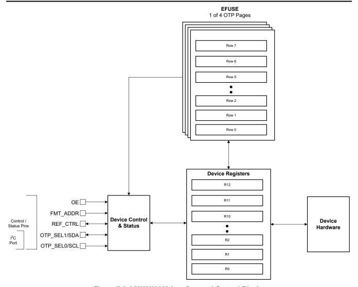
Figure 7-3. LMK3H0102 Interface and Control Blocks
