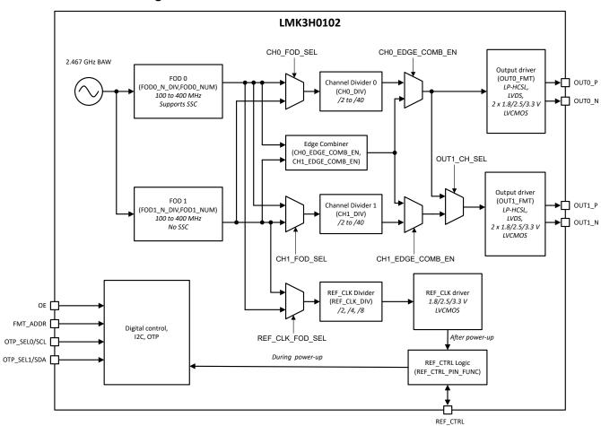
Figure 7-1. LMK3H0102 Functional Block Diagram
