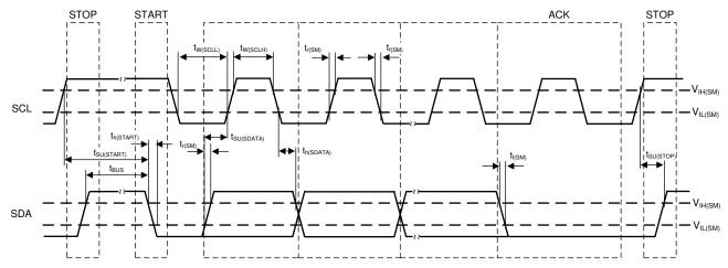
Figure 7-9. I<sup>2</sup>C Timing Diagram
