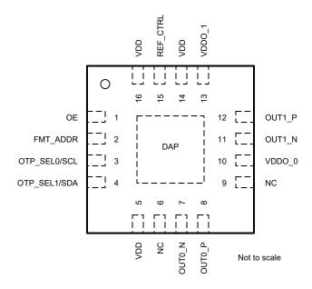
Figure 4-1. LMK3H0102 16-Pin TQFN Top View
