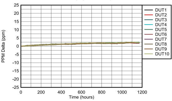
Figure 9-8. Frequency Stability over Time - 1.8V Supply Voltage
