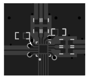
Figure 9-11. PCB Layout Example for LMK3H0102, Top Layer
