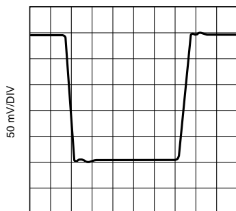
Figure 37. Non-Inverting Large Signal Pulse Response
