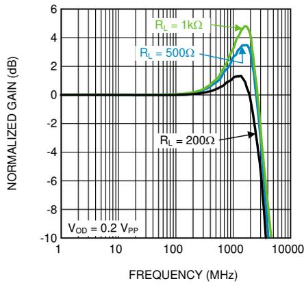
**Figure 5-3. Frequency Response vs  $R_L$**
