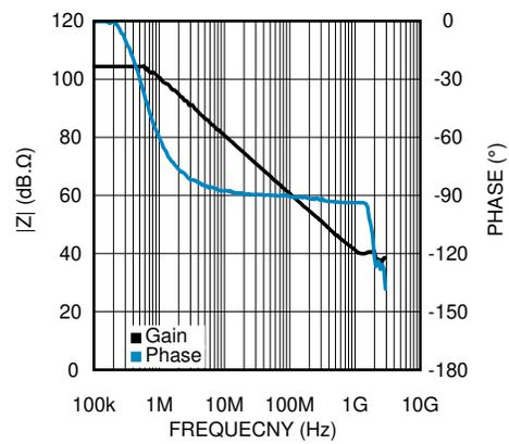
**Figure 5-22. Open Loop Transimpedance**
