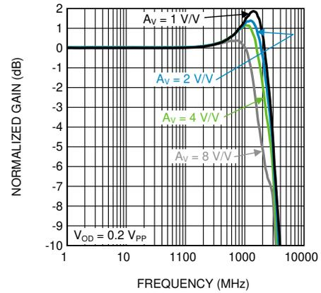
**Figure 5-2. Frequency Response vs Gain**
