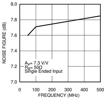
Figure 5-15. Noise Figure vs Frequency
