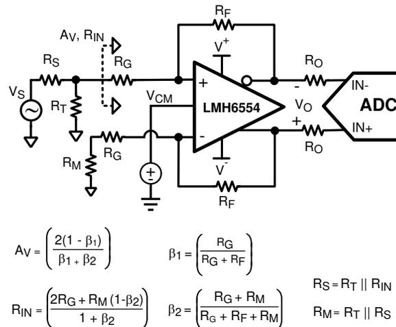
**Figure 7-3. Single-Ended Input with Differential Output**
