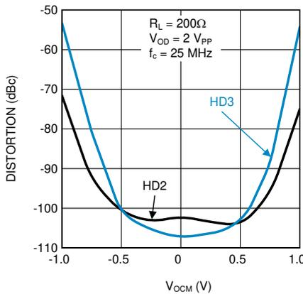
Figure 5-9. Distortion vs Output Common Mode Voltage
