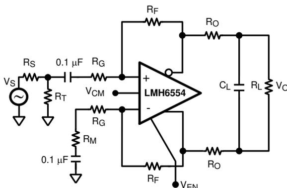
**Figure 7-7. AC Coupled for Single Supply Operation**
