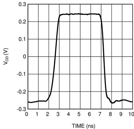
**Figure 5-5.  $0.5\text{ V}_{PP}$  Pulse Response Single-Ended Input**
