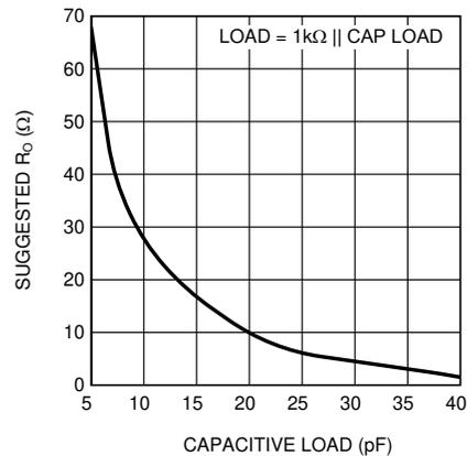
**Figure 7-5. Suggested  $R_{OUT}$  vs Capacitive Load**
