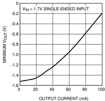
Figure 5-17. Minimum  $V_{OUT}$  vs  $I_{OUT}$
