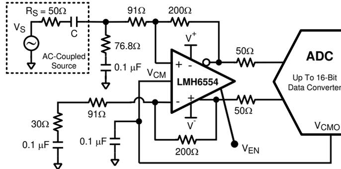
Figure 7-8. Driving a 10-bit Gigasample ADC
