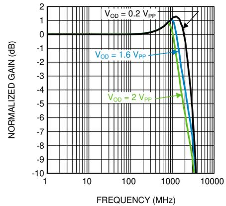
**Figure 5-4. Frequency Response vs Output Voltage ( $V_{OD}$ )**
