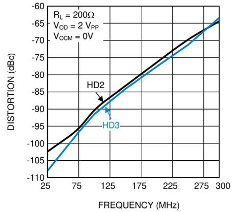
Figure 5-8. Distortion vs Frequency Single-Ended Input
