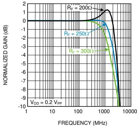
**Figure 5-1. Frequency Response vs  $R_F$**
