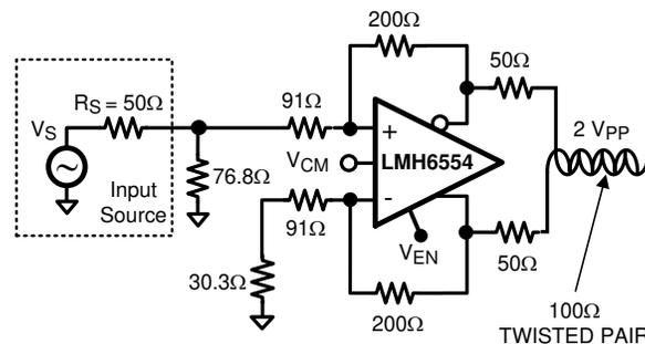
Figure 7-11. Fully Differential Cable Driver
