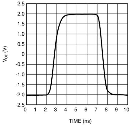
Figure 5-7. 4 V<sub>PP</sub> Pulse Response Single-Ended Input
