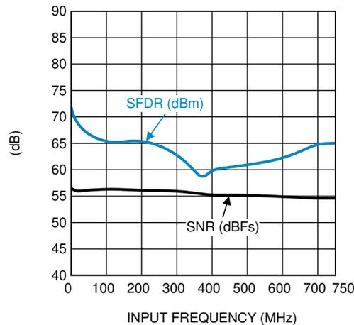
Figure 7-9. LMH6554 / ADC10D1500 SFDR and SNR Performance vs. Frequency
