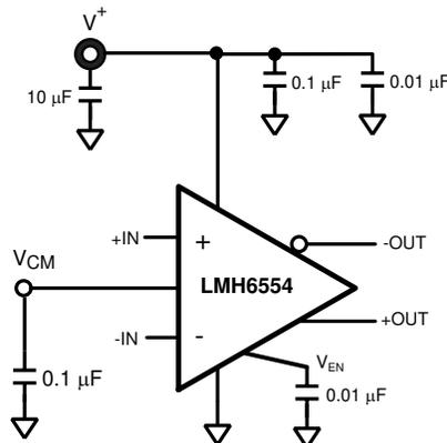
**Figure 7-13. Single Supply Bypassing Capacitors**
