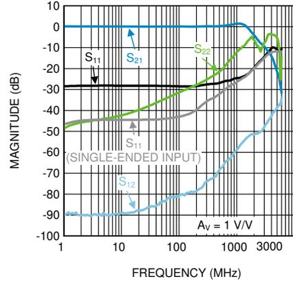
**Figure 5-24. Differential S-Parameter Magnitude vs Frequency**
