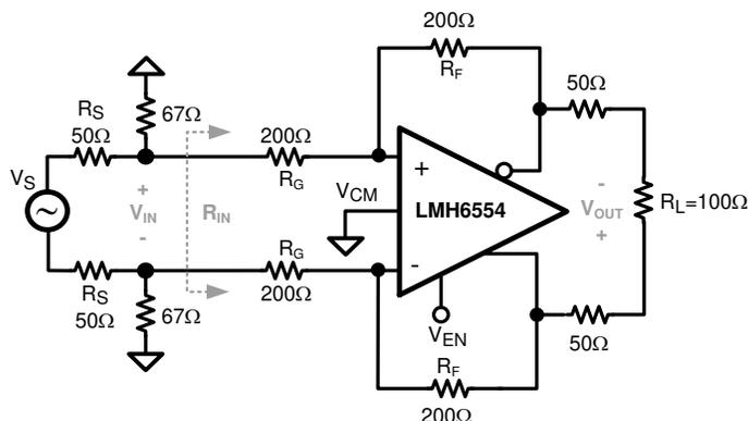
**Figure 7-6. Differential S-Parameter Test Circuit**
