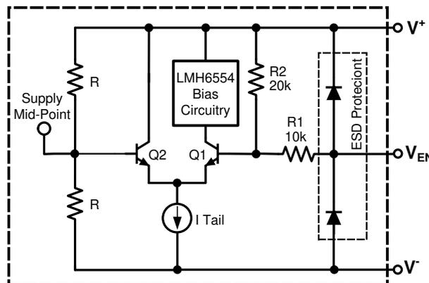
Figure 7-2. Enable Block Diagram
