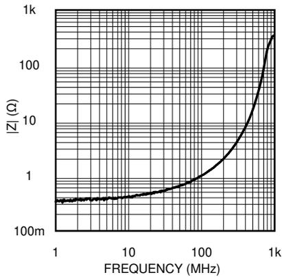
**Figure 5-23. Closed-Loop Output Impedance**
