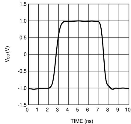
**Figure 5-6.  $2\text{ V}_{PP}$  Pulse Response Single-Ended Input**
