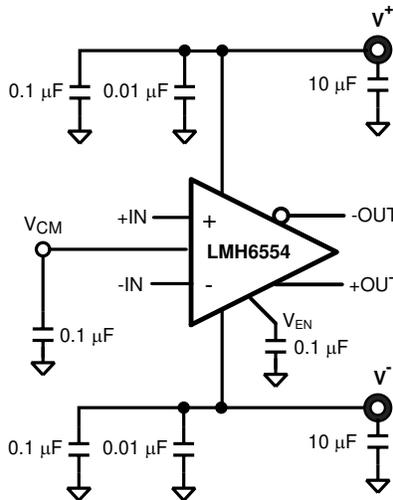
**Figure 7-12. Split Supply Bypassing Capacitors**
