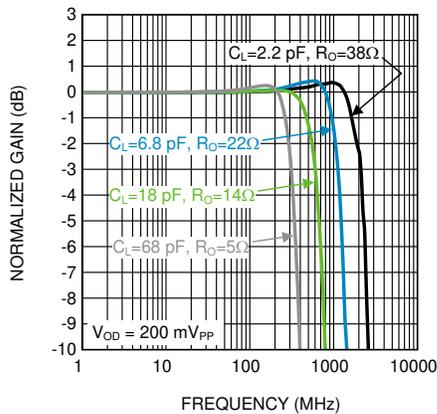
**Figure 7-4. Frequency Response vs Capacitive Load**
