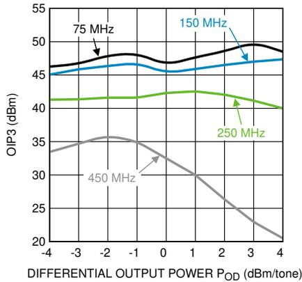
Figure 5-13. OIP3 vs Output Power  $P_{OUT}$
