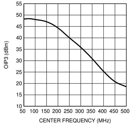
Figure 5-14. OIP3 vs Center Frequency
