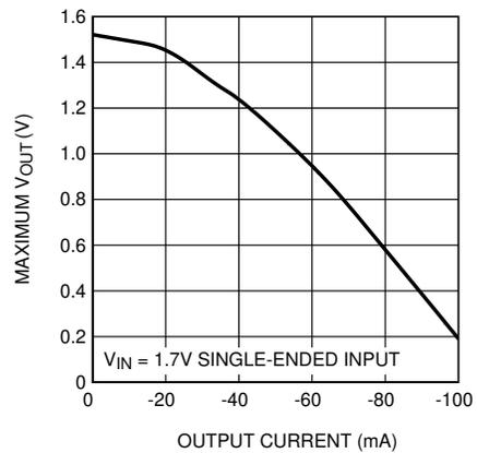
Figure 5-16. Maximum  $V_{OUT}$  vs  $I_{OUT}$
