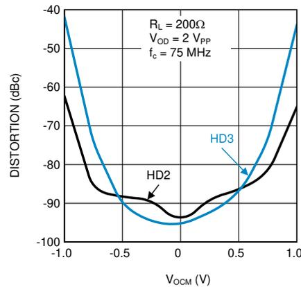
Figure 5-10. Distortion vs Output Common Mode Voltage
