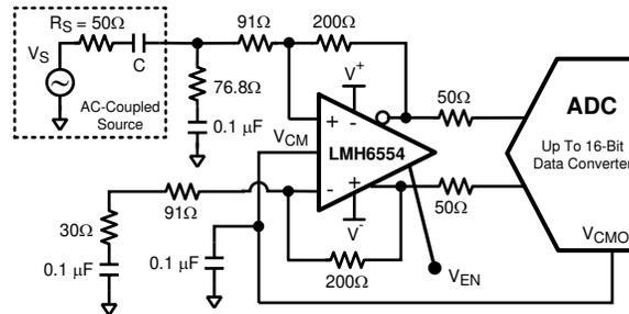
Figure 7-1. Single-Ended Input to Differential Output Schematic
