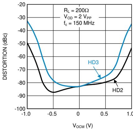
Figure 5-11. Distortion vs Output Common Mode Voltage
