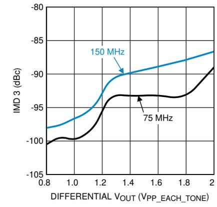
Figure 5-12. 3rd Order Inter-Modulation Products vs V<sub>OUT</sub>
