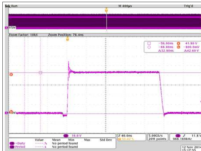
Figure 12. SW Node Behavior Showing the Dead Time
