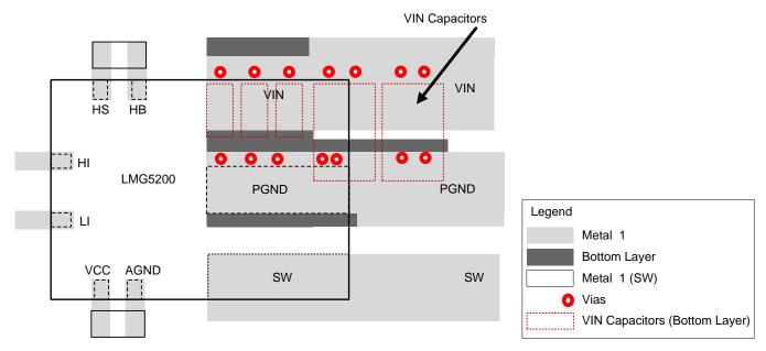
Figure 20. External Component Placement (Double Layer PCB)
