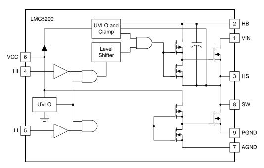
Figure 10. Functional Block Diagram
