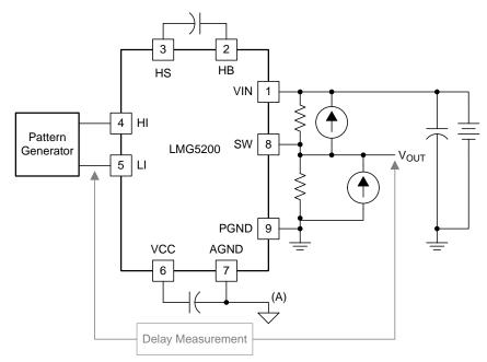
Figure 5. Propagation Delay and Propagation Mismatch Measurement
