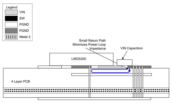
Figure 15. Four-Layer Board Cross Section With Return Path Directly Underneath for Power Loop
