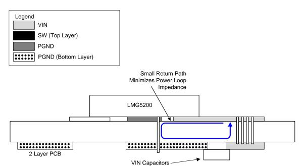
Figure 21. Two-Layer Board Cross Section With Return Path
