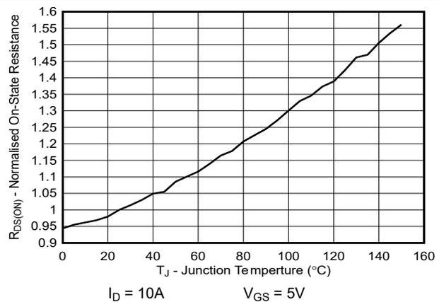
Figure 5-6. LMG3100R017 Normalized On-State Resistance vs Junction Temperature
