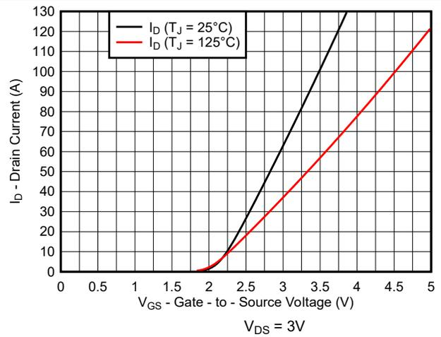
Figure 5-10. LMG3100R044 Typical Transfer Characteristics
