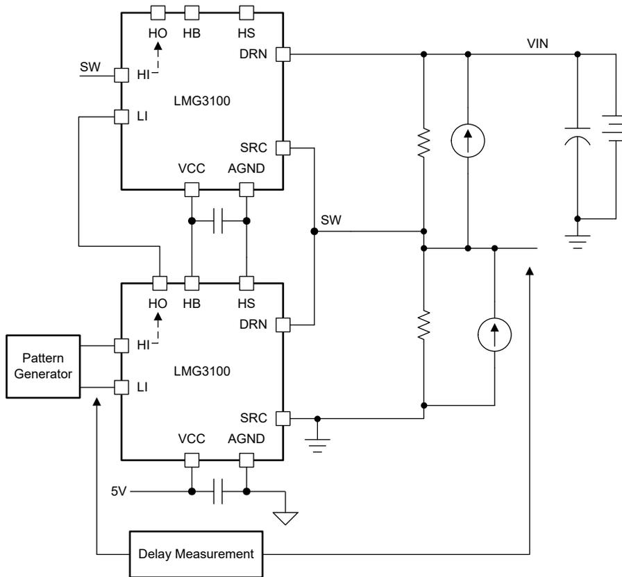
**Figure 6-1. Propagation Delay and Propagation Mismatch Measurement**
