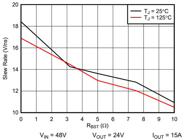
**Figure 5-15. LMG3100R044 Slew Rate Control for a Buck Converter Using R<sub>BST</sub>**
