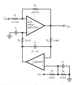
Figure 55. High Gain Amplifier with Low Frequency Null
