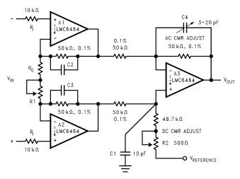
Figure 47. Low Power Three Op-Amp Instrumentation Amplifier
