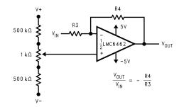
Figure 40. Inverting Configuration, Offset Voltage Adjustment
