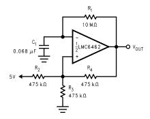
Figure 54. 1 Hz Square-Wave Oscillator
