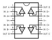
Figure 1. 14-Pin CDIP Top View
