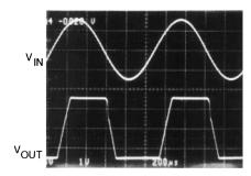
Figure 33. A ±7.5V Input Signal Greatly Exceeds the 3V Supply in Figure 34 Causing No Phase Inversion Due to R<sub>1</sub>
