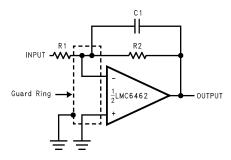
Figure 43. Inverting Amplifier
