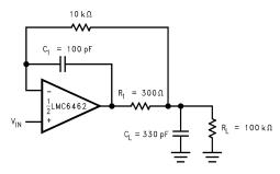
Figure 37. LMC6464 Non-Inverting Amplifier, Compensated to Handle a 300 pF Capacitive and 100 KΩ Resistive Load
