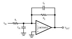
Figure 39. Canceling the Effect of Input Capacitance
