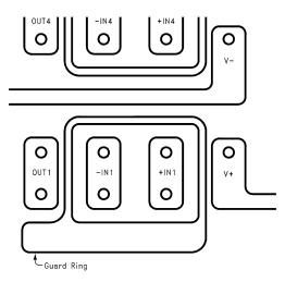
Figure 42. Example of Guard Ring in P.C. Board Layout
