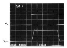
Figure 38. Pulse Response of LMC6464 Circuit in Figure 37
