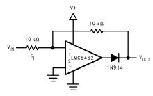
Figure 52. Full-Wave Rectifier with Input Current Protection (R<sub>I</sub>)
