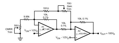
Figure 2. Low-Power Two-Op-Amp Instrumentation Amplifier
