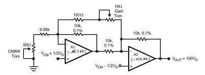
Figure 48. Low-Power Two-Op-Amp Instrumentation Amplifier
