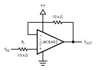
Figure 51. Half-Wave Rectifier with Input Current Protection (R<sub>I</sub>)
