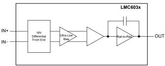
Figure 6-1. LMC603x Circuit Topology (Each Amplifier)
