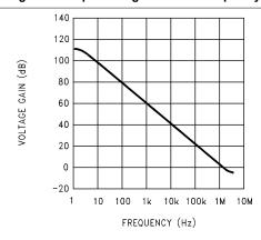
Figure 5-10. Open-Loop Frequency Response
