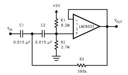
Typical Application: 10Hz High-Pass Filter
