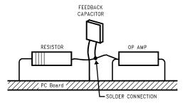
Input pins are lifted out of PCB and soldered directly to components. All other pins connected to the PCB.
