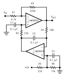
Gain = -46.8 Output offset voltage reduced to the level of the input offset voltage of the bottom amplifier (typically 1mV).
