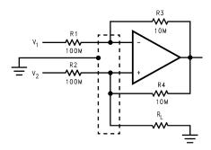
Figure 6-20. Howland Current-Pump Guard-Ring Connections
