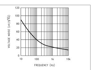
Figure 5-8. Input Voltage Noise vs Frequency
