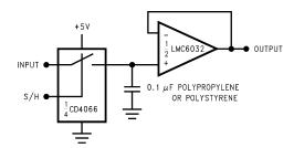
Figure 6-9. Low-Leakage Sample-and-Hold
