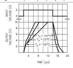
Figure 5-12. Noninverting Large-Signal Pulse Response
