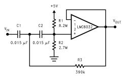
$f_c$  = 10Hz, d = 0.895, gain = 1, 2dB pass-band ripple
