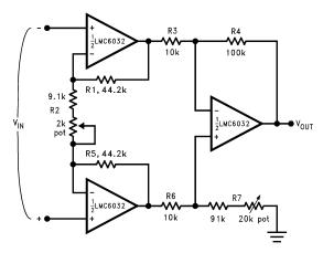
Figure 6-6. Instrumentation Amplifier
