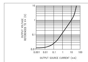
Figure 5-7. Output Characteristics Current Sourcing
