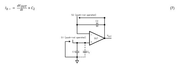
Figure 6-5. Simple Input Bias Current Test Circuit
