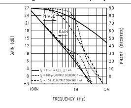
Figure 5-11. Frequency Response vs Capacitive Load
