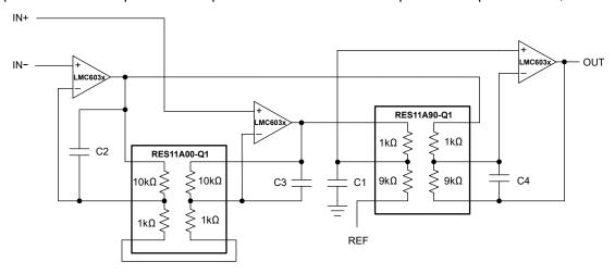
Figure 6-7. Improved Instrumentation Amplifier With RES11A
