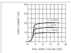
Figure 5-1. Supply Current vs Supply Voltage
