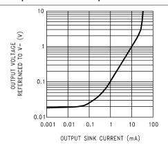
Figure 5-6. Output Characteristics Current Sinking
