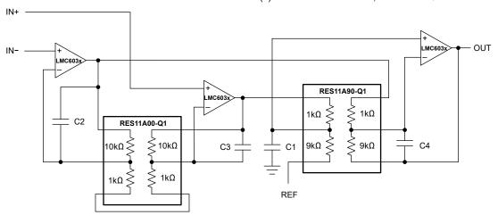
Typical Application: Instrumentation Amplifier With RES11A
