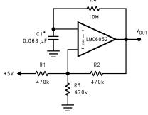
Figure 6-10. 1Hz Square-Wave Oscillator
