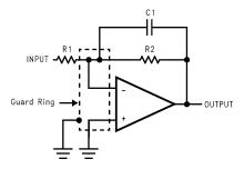
Figure 6-17. Inverting Amplifier Guard-Ring Connections
