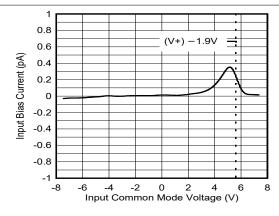
Figure 5-4. Input Bias Current vs Input Common-Mode Voltage
