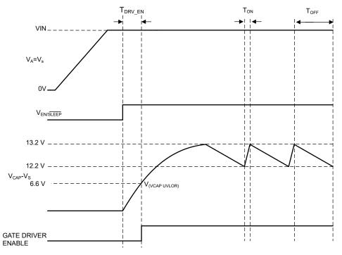
Figure 8-1. Charge Pump Operation
