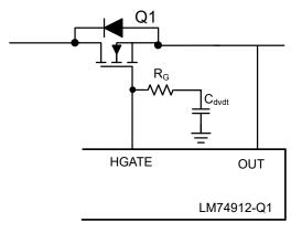
Figure 8-2. Inrush Current Limiting
