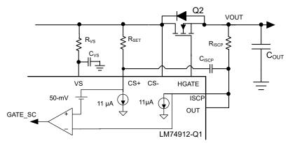
Figure 8-4. Short Circuit Protection With De-glitch Filter
