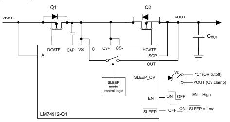
Figure 8-7. Extending Overvoltage Threshold in SLEEP Mode
