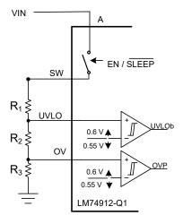
Figure 8-5. Programming Overvoltage Threshold and Battery Sensing
