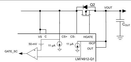
Figure 8-3. Short Circuit Protection Comparator
