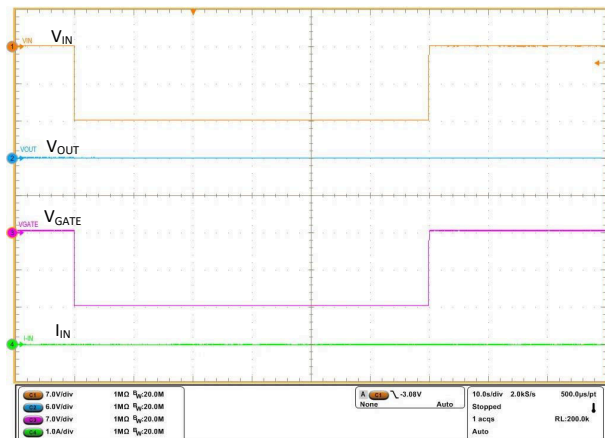
Figure 9-9. Reverse Input Voltage -14 V for 60 s
