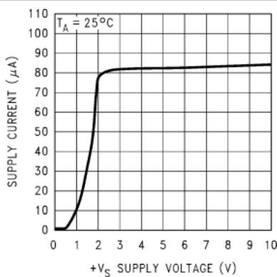
**Figure 6-17. Supply Current vs Supply Voltage (Legacy chip)**
