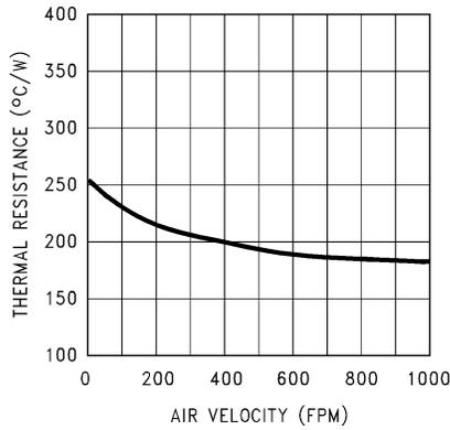
Figure 6-1. Thermal Resistance Junction to Air (Legacy chip)
