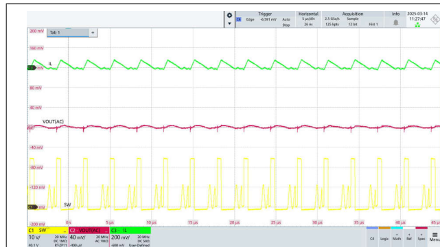
Figure 7-8. DCM Steady State Ripple
