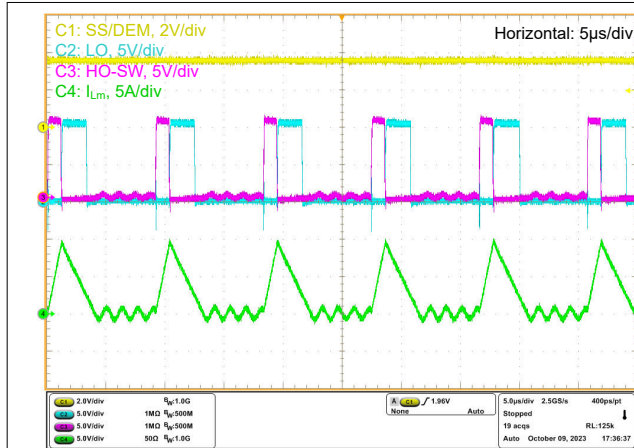
Figure 7-24. DEM: Buck Mode, I_{load} = 4A
