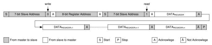
Figure 6-37. Sequential READ Starting From A Defined Register Address
