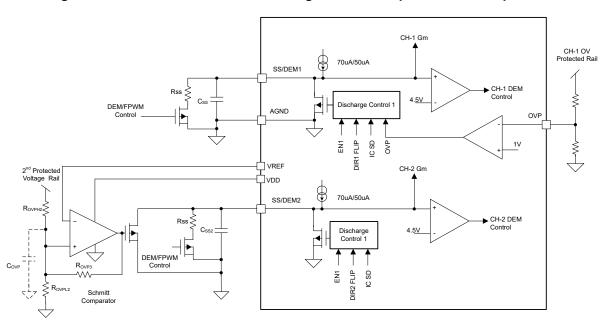
Figure 6-24. Independent Channel Operation OVP Implementation
