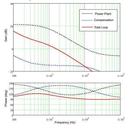
Figure 7-12. Bode Plots of the Voltage Loop
