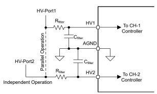
Figure 6-2. HV1 and HV2 Pins Configuration
