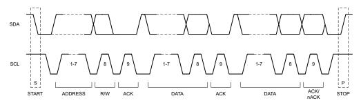
Figure 6-33. I <sup>2</sup> C START / STOP / ACKNOWLEDGE Protocol
