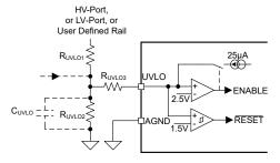
Figure 6-32. UVLO With Additional Hysteresis Programming
