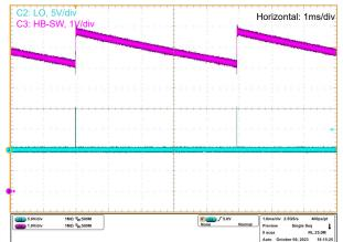
Figure 7-29. Pre-charge: Buck Mode, I<sub>load</sub>= 0A
