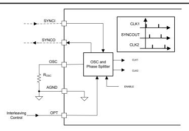
Figure 6-21. Oscillator and Interleaving Clock Programming
