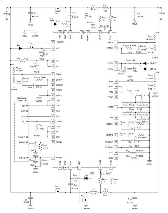
Figure 7-7. Schematic of the Example Dual-Phase Bidirectional Converter
