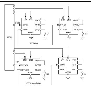
Figure 6-27. Eight Phases 45° Interleaving Configuration using External Clock Shift
