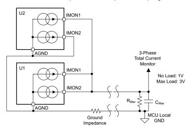
Figure 6-8. An Example of the 3-Phase Total Inductor Current Monitor
