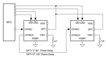
Figure 6-25. Three or Four Phases Interchangeable Configuration
