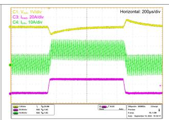
Figure 7-18. Step Load Response: Buck Mode; FPWM; 1A to 30A Load Step; 1A/µs
