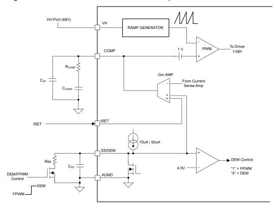
Figure 6-10. Inner Loop GM Amplifier, Soft-Start, and PWM Comparator, and DEM/FPWM Control
