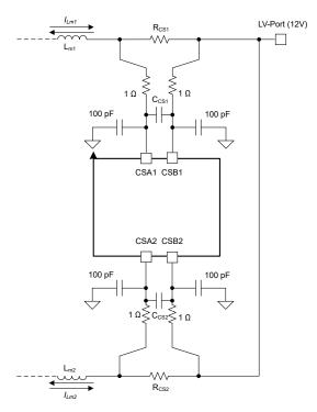
Figure 7-8. Current Sense With RC filter
