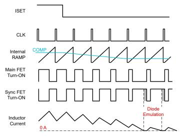
Figure 6-11. Diode Emulation Operation
