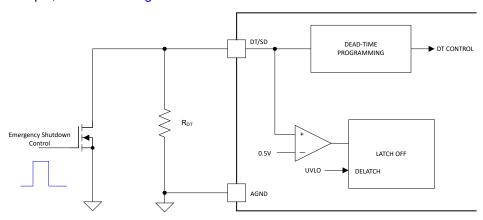
Figure 6-19. Emergency Latched Shutdown
