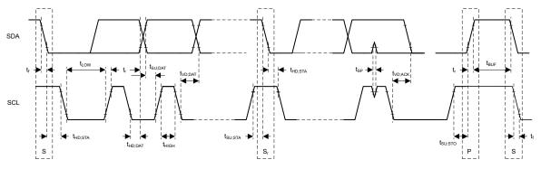
Figure 6-34. I <sup>2</sup> C Data Transmission Timing
