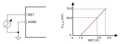
Figure 6-3. Analog Voltage Channel Current Programming
