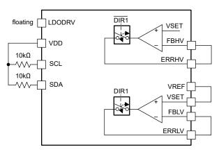
Figure 7-14. Proper Termination of Unused Pins
