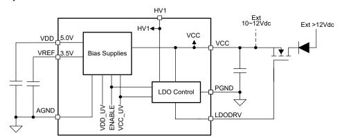
Figure 6-1. Bias Supplies Connections
