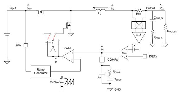
Figure 7-1. Buck Loop Block Diagram
