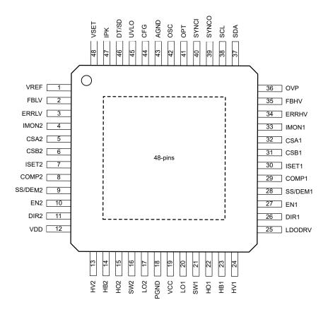
Figure 4-1. PHP Package 48-Pin TQFP Top View
