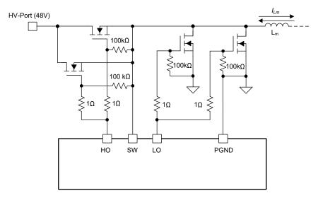
Figure 7-9. Paralleled MOSFET Configuration
