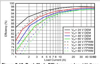
Figure 7-15. Buck Mode Efficiency vs Input Voltage and Load Current: V<sub>OUT</sub> = 14.5V
