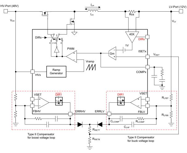
Figure 7-6. Outer Voltage Loop Control
