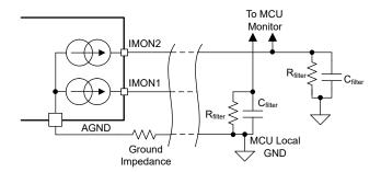
Figure 6-7. Channel Current Monitor
