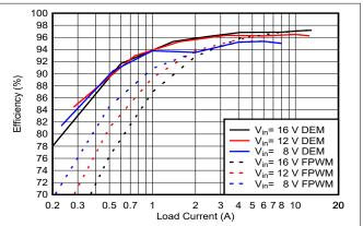
Figure 7-16. Boost Mode Efficiency vs Input Voltage and Load Current: V<sub>OUT</sub> = 50.5V
