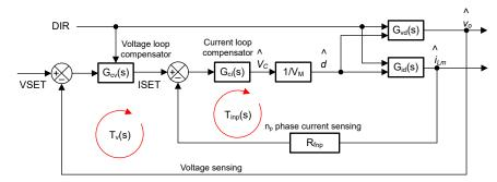
Figure 7-5. Voltage Loop and Current Loop Block Diagram
