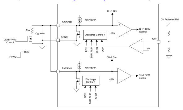
Figure 6-12. OVP Implementation for SS-DEM Pins Connection for Parallel Operation
