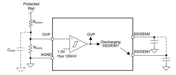
Figure 6-22. OVP for CH-1 or Multiphase Parallel Operation
