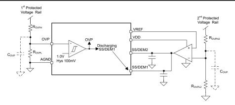
Figure 6-23. OVP for 2nd Protected Voltage Rail in Multiphase Parallel Operation
