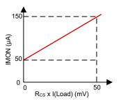
Figure 6-6. IMON Current Source vs Boost Load Current
