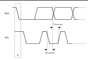
Figure 6-35. I <sup>2</sup> C Data Transmission Timing for maximum rise/fall times.
