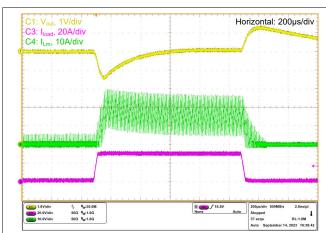
Figure 7-17. Step Load Response: Buck Mode; DEM; 1A to 30A Load Step; 1A/µs
