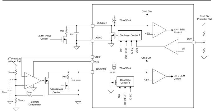
Figure 6-13. OVP Implementation for Independent Channel Operation
