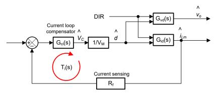
Figure 7-2. Current Loop Block Diagram
