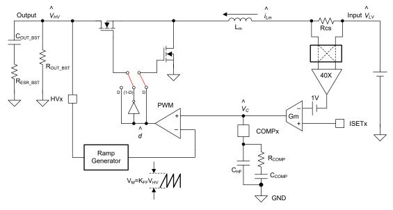
Figure 7-3. Boost Loop Block Diagram
