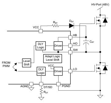
Figure 6-15. Dead Time Programming With DT Pin (Only One Channel is Shown)
