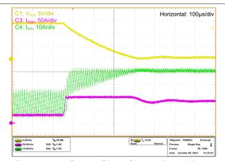
Figure 7-31. Output Short Circuit: Buck Mode
