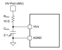
Figure 7-10. HVx Pin Configuration
