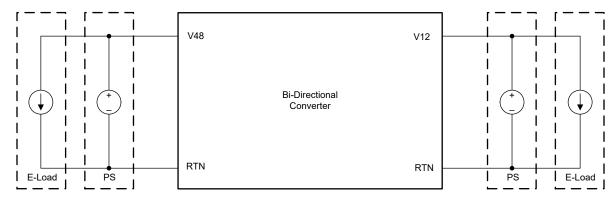
Figure 7-32. Emulated Dual Battery System With Bench Power Supplies and E-Loads
