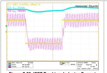
Figure 7-28. ISET Tracking: Inductor Current Tracking with Direction Change
