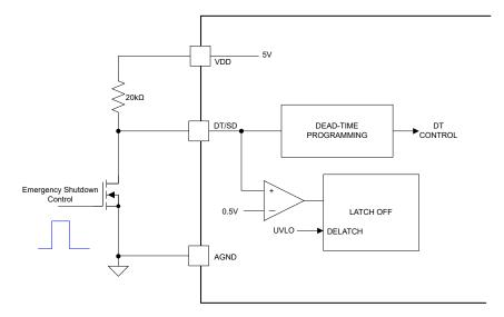
Figure 6-20. Emergency Latched Shutdown with Adaptive Deadtime Scheme
