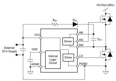
Figure 6-14. Bootstrap Circuit for High-Side Bias Supply (Only One Channel is Shown)
