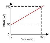
Figure 6-5. IMON Current Source vs Current Sense Voltage
