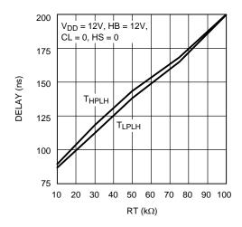
Figure 17. Turn On Delay vs RT Resistor Value
