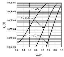
Figure 7. Diode Forward Voltage
