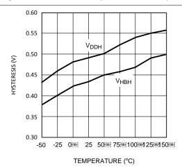
Figure 8. Undervoltage Threshold Hysteresis vs Temperature
