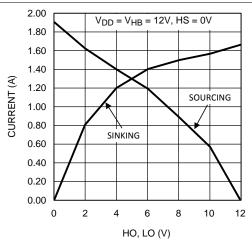
Figure 6. HO & LO Peak Output Current vs Output Voltage
