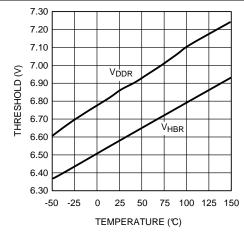
Figure 9. Undervoltage Rising Threshold vs Temperature
