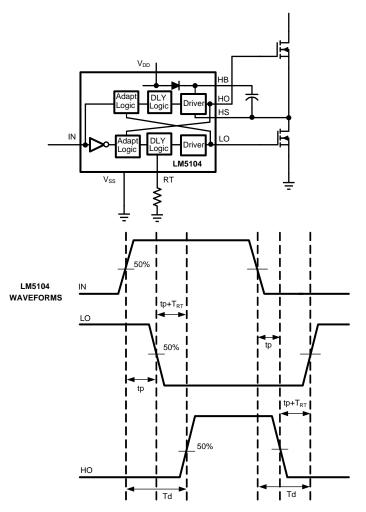
Figure 16. Application Timing Waveforms
