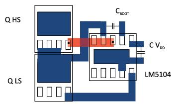
Figure 21. LM5104 Component Placement
