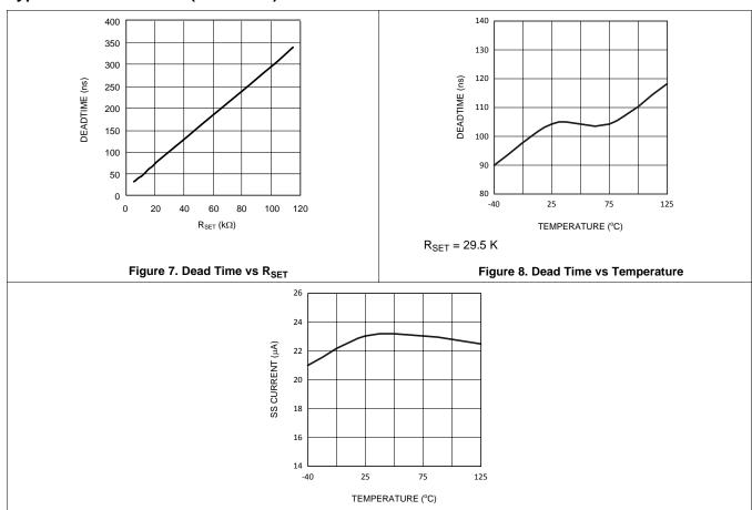
Figure 9. SS Pin Current vs Temperature
