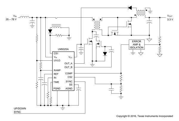
Figure 14. Simplified Active Clamp Forward Power Converter
