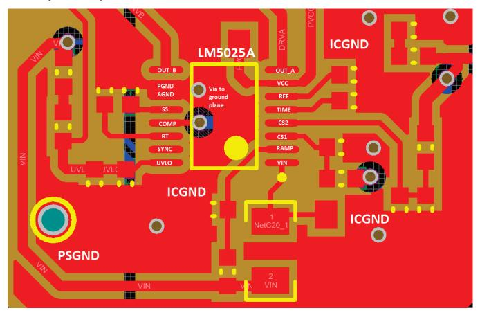
Figure 23. LM5025A Layout Recommendation
