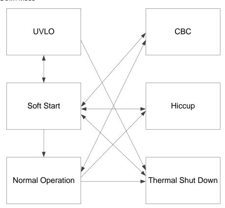
Figure 13. Functional Mode Transition Diagram
