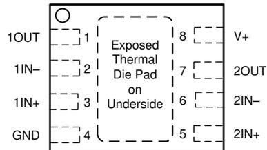
Connect thermal pad directly to GND pin.
