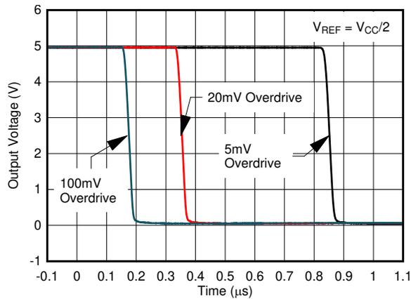
**Figure 5-31. Response Time for Various Overdrives, High-to-Low Transition**
