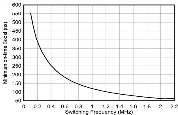
Figure 6-21. Boost Minimum On-time versus Switching Frequency
