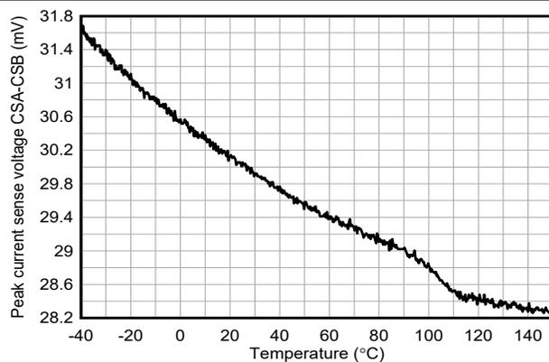
**Figure 6-29. Average Current Limit Threshold Voltage Versus Temperature
