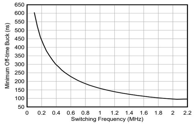
Figure 6-18. Buck Minimum Off-time versus Switching Frequency
