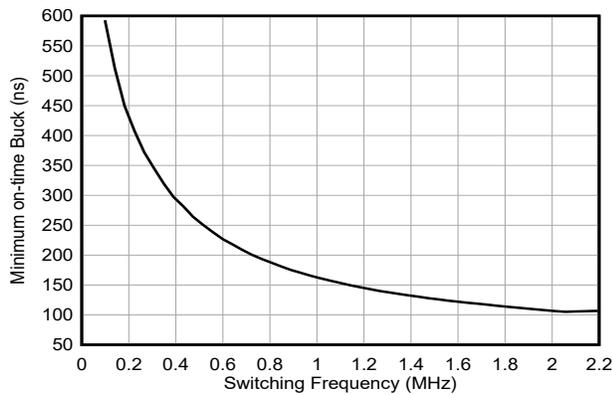
Figure 6-19. Buck Minimum On-time versus Switching Frequency
