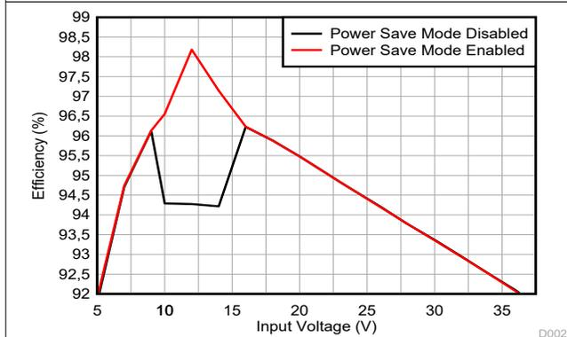
Figure 10-4. Efficiency Versus  $V_I$  ( $V_O = 12V$ ,  $I_O = 5A$ )
