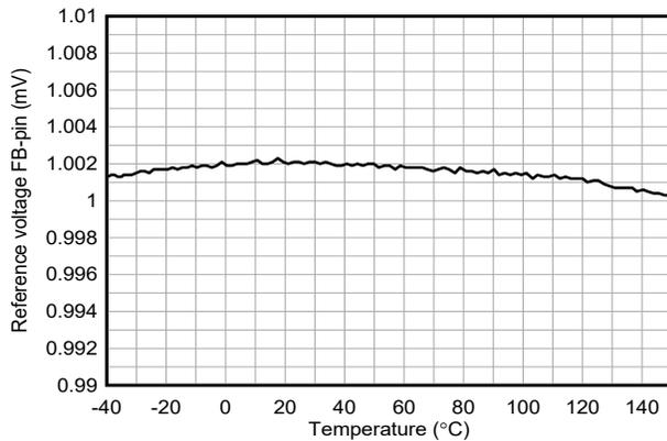
**Figure 6-3. FB Pin Reference Voltage versus Temperature**
