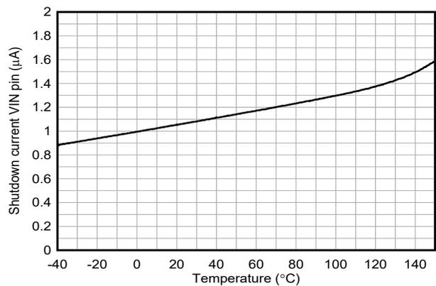
**Figure 6-6. Shutdown Current into VIN versus Temperature**
