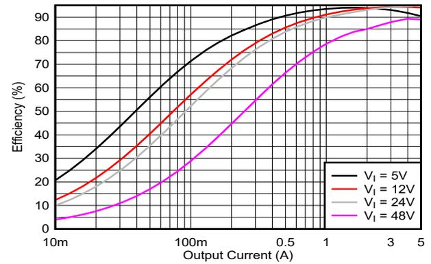
Figure 10-3. Efficiency Versus  $I_O$  (MODE = VCC2,  $V_O = 12V$ )
