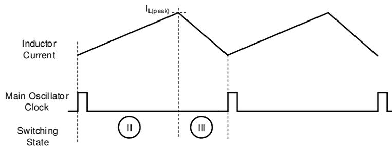
**Figure 8-3. Inductor Current in Continuous Current Buck Operation**
