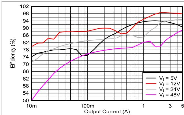
Figure 10-2. Efficiency Versus  $I_O$  (MODE = 0V,  $V_O = 12V$ )
