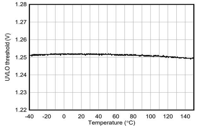
Figure 6-16. EN/UVLO Threshold versus Temperature
