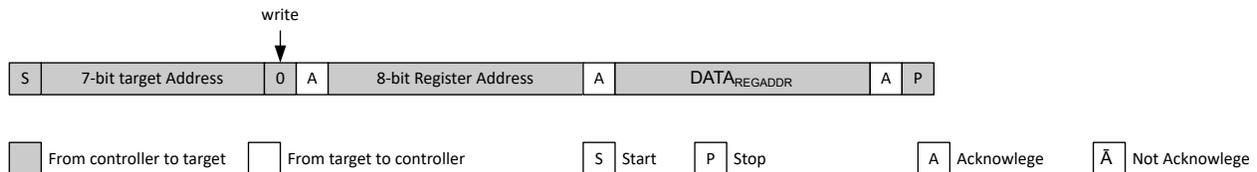
Figure 8-38. Single WRITE to Defined Register Address
