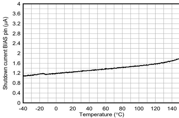
**Figure 6-7. Shutdown Current into BIAS versus Temperature**
