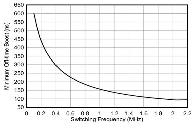
Figure 6-20. Boost Minimum Off-time versus Switching Frequency
