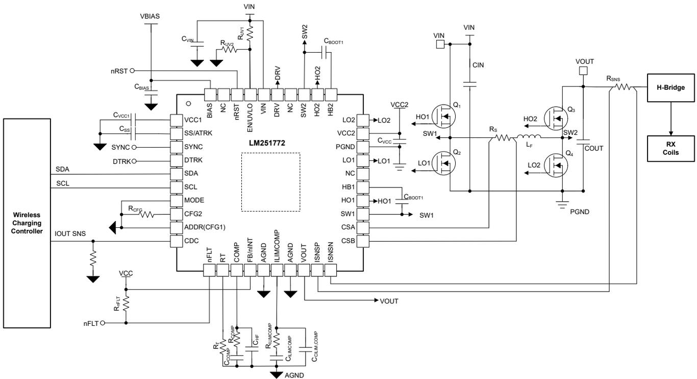
Figure 10-27. Simplified Schematic of a Wireless Charging Supply
