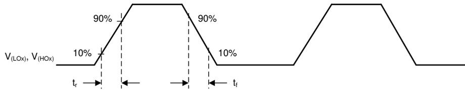
Figure 7-1. Timing Diagram Gate Driver  $t_r$ ,  $t_f$
