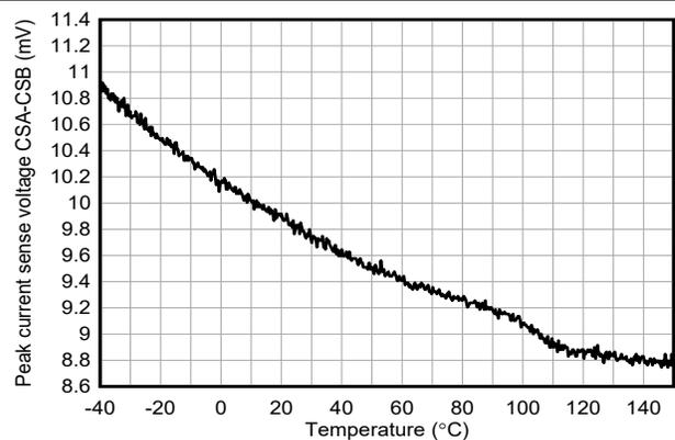
**Figure 6-30. Average Current Limit Threshold Voltage Versus Temperature
