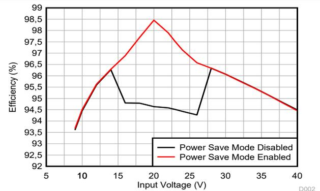
Figure 10-5. Efficiency Versus  $V_I$  ( $V_O = 20V$ ,  $I_O = 5A$ )
