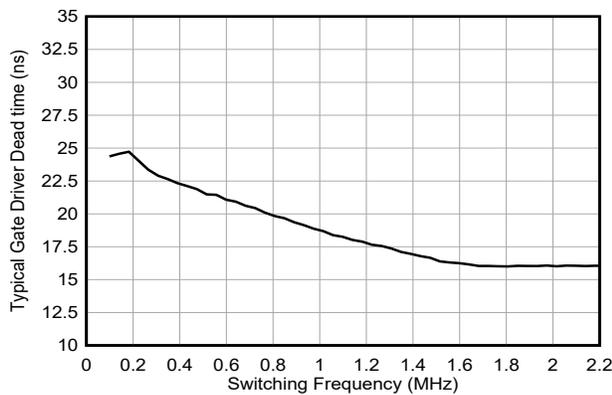
Figure 6-23. Gate Driver Transition (Dead) Time versus Switching Frequency
