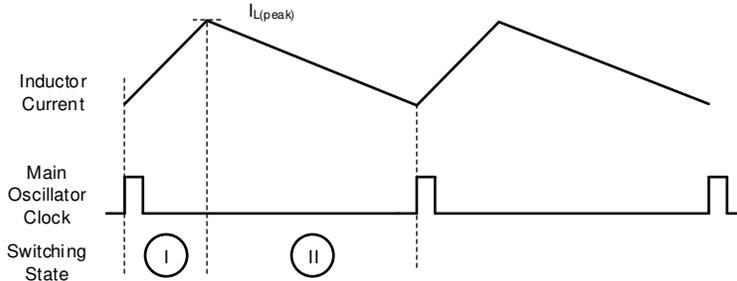
**Figure 8-4. Inductor Current in Continuous Current Boost Operation**
