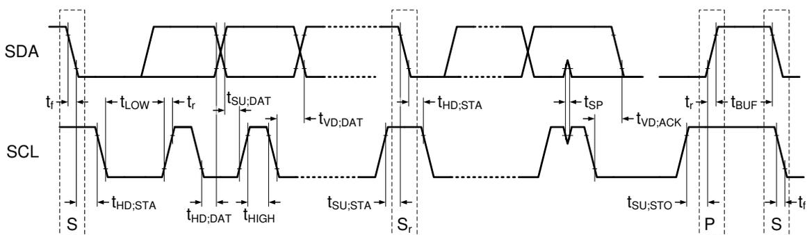
**Figure 8-34. I<sup>2</sup>C Data Transmission Timing**
