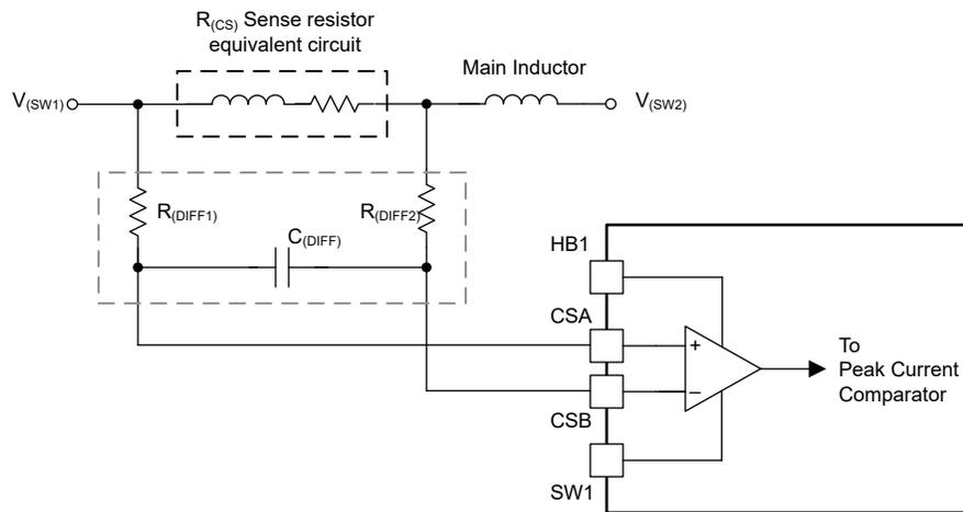
**Figure 8-17. Simplified Schematic of the Peak Current Sensor**
