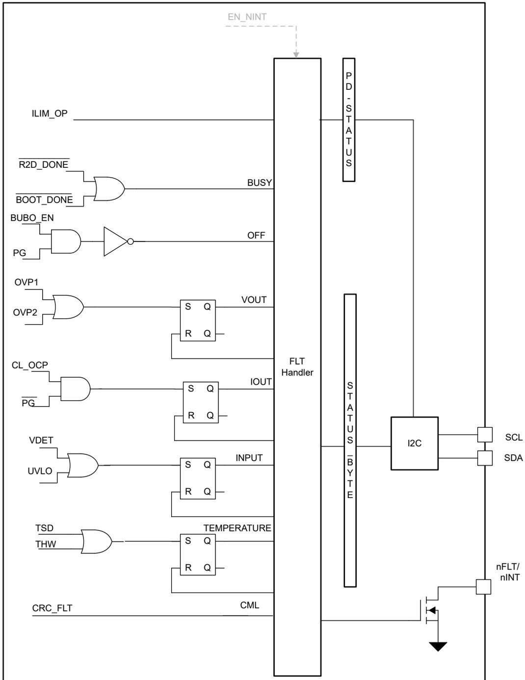
Figure 8-29. Functional Block Diagram Fault Handler
