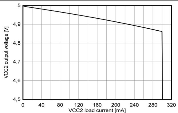
**Figure 6-12. VCC2 LDO Output voltage versus VCC2 Load Current**
