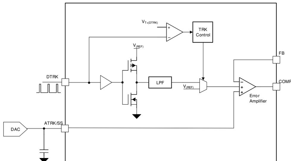
**Figure 8-24. Output Voltage Tracking Functional Block Diagram**
