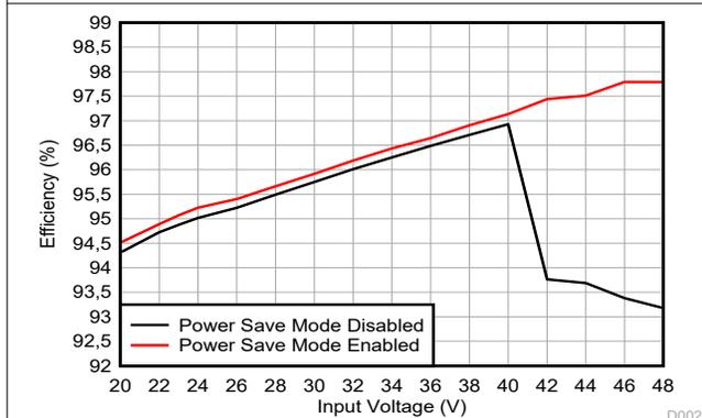
Figure 10-6. Efficiency Versus  $V_I$  ( $V_O = 48V$ ,  $I_O = 5A$ )
