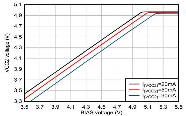
Figure 6-14. VCC2 LDO Output voltage versus BIAS Voltage
