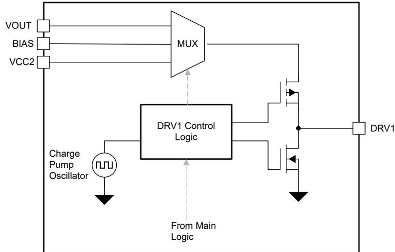
**Figure 8-25. Functional Block Diagram - DRV pin**
