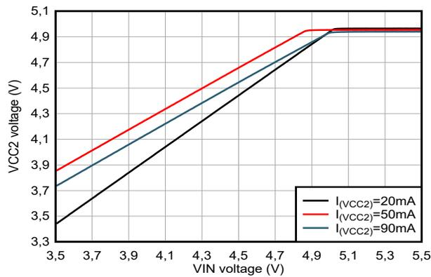
Figure 6-13. VCC2 LDO Output voltage versus VIN Voltage
