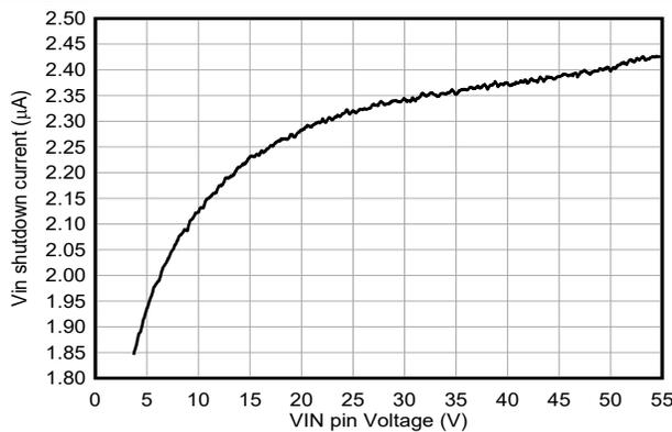
**Figure 6-5. Shutdown Current into VIN versus Pin Voltage**
