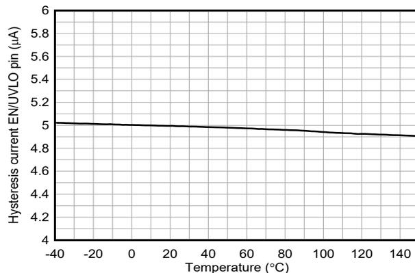
Figure 6-17. Hysteresis Current on EN/UVLO versus Temperature
