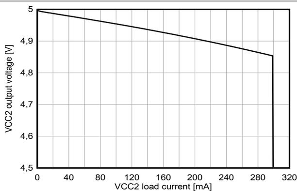
**Figure 6-11. VCC2 LDO Output voltage versus VCC2 Load Current**
