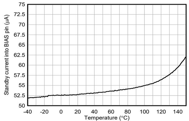
**Figure 6-10. Standby Current into BIAS versus Temperature**
