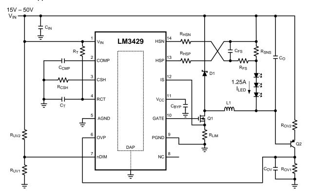
Figure 35. Buck Application - 3 LEDS at 1.25 A Schematic
