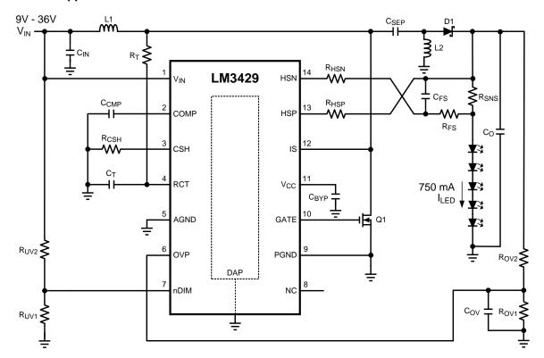
Figure 37. 5 LEDs at 750 mA
