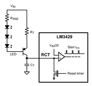
Figure 14. Off-timer Circuitry for Buck Regulators
