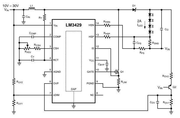
Figure 32. Buck-Boost Analog Dimming Application - 4 LEDs at 2 A Schematic
