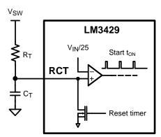
Figure 13. Off-timer Circuitry for Boost and Buck-boost Regulators
