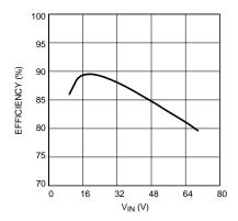
Figure 30. Buck-Boost Efficiency vs Input Voltage, V<sub>O</sub>= 6 LEDs
