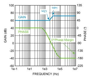
Figure 18. Uncompensated Loop Gain Frequency Response
