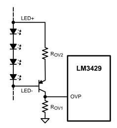
Figure 22. Floating Output OVP Circuitry
