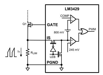
Figure 17. Current Sense / Current Limit Circuitry
