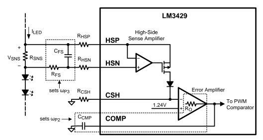
Figure 19. Compensation Circuitry
