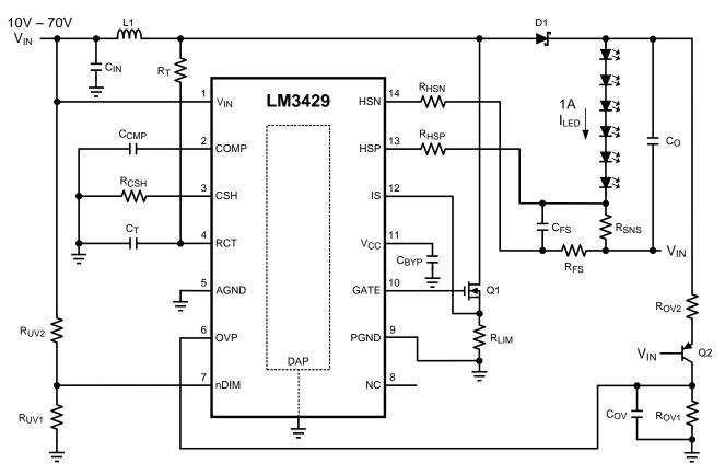
Figure 29. Buck-Boost Application - 6 LEDs at 1 A Schematic
