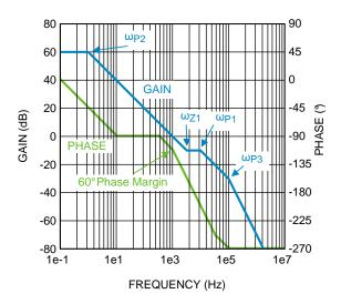
Figure 20. Compensated Loop Gain Frequency Response
