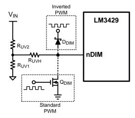
Figure 24. PWM Dimming Circuit
