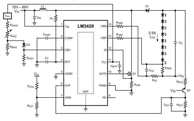
Figure 36. Buck-Boost Thermal Foldback Application - 8 LEDs at 2.5 A Schematic
