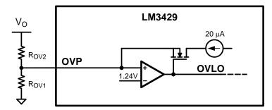
Figure 21. Overvoltage Protection Circuitry
