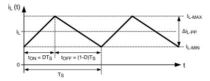
Figure 12. Ideal CCM Regulator Inductor Current i<sub>L</sub>(t)
