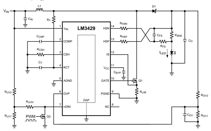
Figure 26. Boost Regulator  $(V_{IN} < V_{O})$
