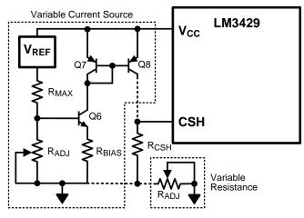
Figure 16. Analog Dimming Circuitry
