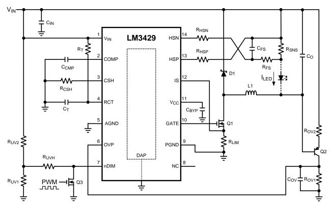
Figure 27. Buck Regulator  $(V_{IN} > V_O)$
