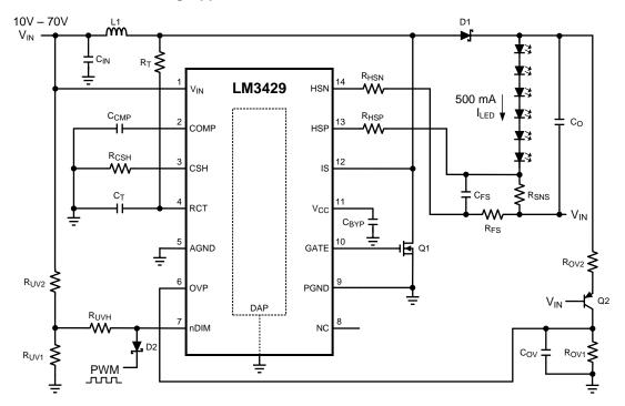
Figure 34. Buck-Boost PWM Dimming Application - 6 LEDs at 500 mA
