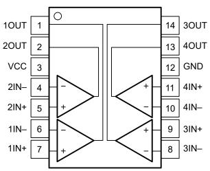
Figure 4-1. D, N Packages 14-Pin SOIC, PDIP Top View
