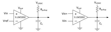
Figure 7-1. Single-ended and Differential Comparator Configurations
