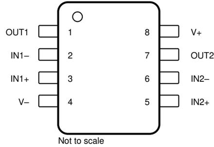
**Figure 5-2. LM358LV D, DGK, PW, and DDF Package
