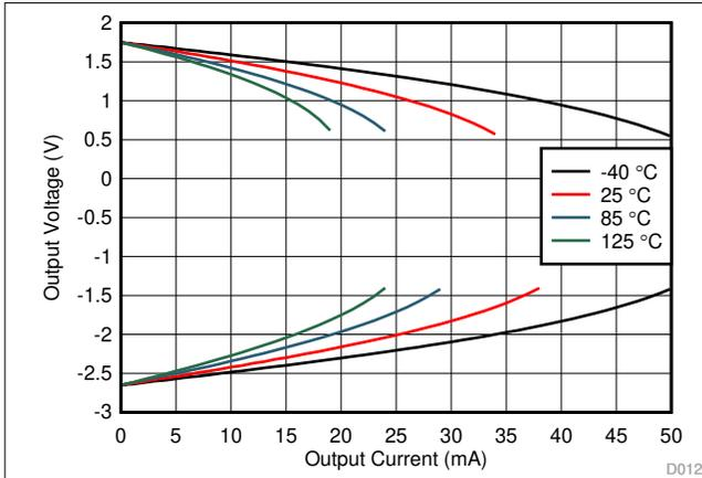
**Figure 6-6. Output Voltage vs Output Current (Claw)**
