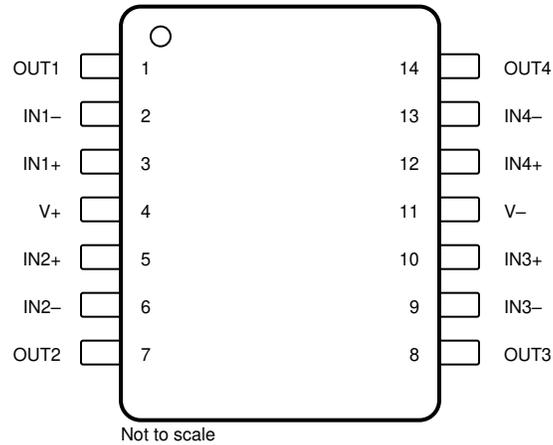
**Figure 5-3. LM324LV D, PW, and DYY Package
