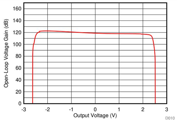
**Figure 6-4. Open-Loop Voltage Gain vs Output Voltage**
