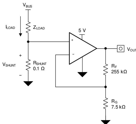
Figure 8-1. LM3xxLV Device in a Low-Side, Current-Sensing Application
