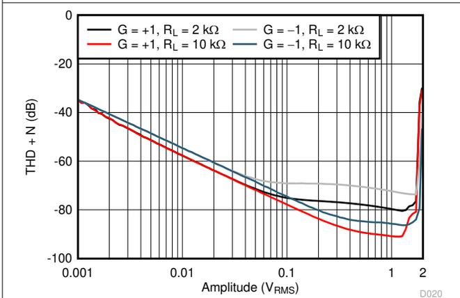
$V_S = 5.5\text{ V}$        $V_{CM} = 2.5\text{ V}$        $G = 1$
