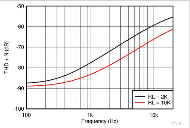
$V_S = 5.5\text{ V}$        $V_{CM} = 2.5\text{ V}$        $G = 1$
