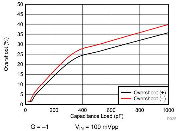
Figure 6-19. Small Signal Overshoot vs Capacitive Load
