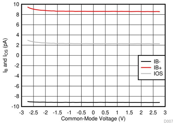
**Figure 6-1.  $I_B$  and  $I_{OS}$  vs Common-Mode Voltage**
