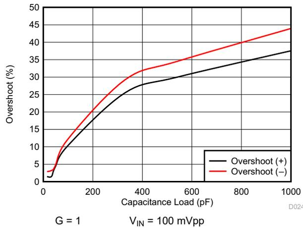
Figure 6-18. Small Signal Overshoot vs Capacitive Load
