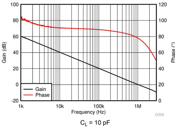
**Figure 6-3. Open-Loop Gain and Phase vs Frequency**
