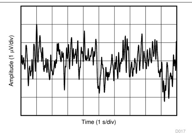
**Figure 6-11. 0.1-Hz to 10-Hz Integrated Voltage Noise**
