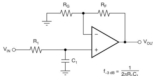
$$\frac{V_{\text{OUT}}}{V_{\text{IN}}} = \left(1 + \frac{R_F}{R_G}\right) \left(\frac{1}{1 + sR_1C_1}\right)$$
