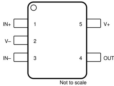
**Figure 5-1. LM321LV DBV and DCK Package
