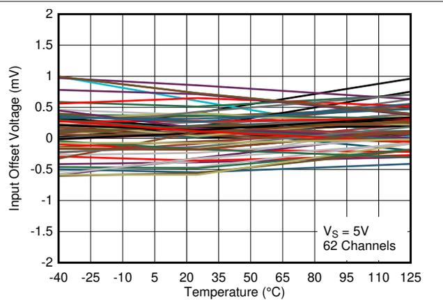
Figure 5-8. Input Offset Voltage vs. Temperature at 5V
