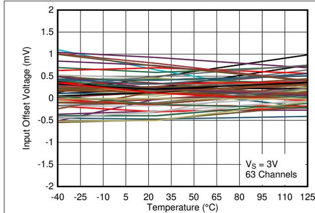
Figure 5-7. Input Offset Voltage vs. Temperature at 3V
