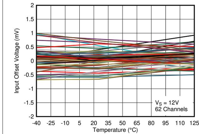
Figure 5-9. Input Offset Voltage vs. Temperature at 12V
