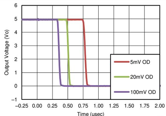
**Figure 4-3. Response Time for Various Overdrives (Negative Transition)**
