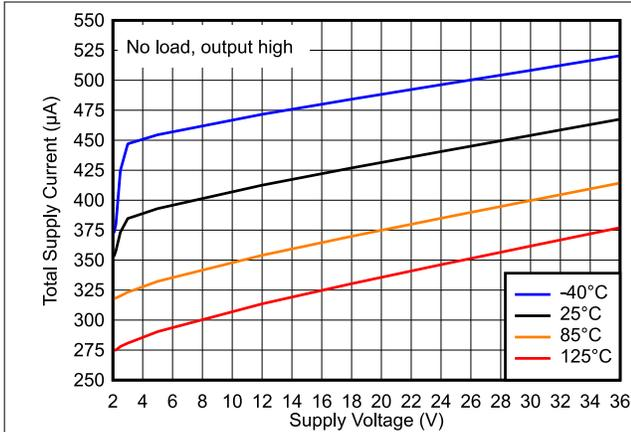
Figure 2-1. Total Supply Current vs. Supply Voltage
