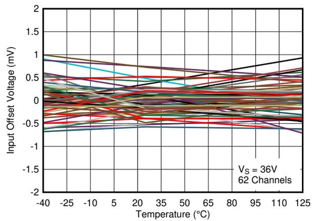
Figure 2-10. Input Offset Voltage vs. Temperature at 36V
