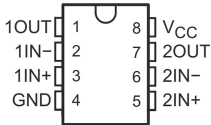
**Figure 1-1. D, DGK, DDF OR PW PACKAGE**
