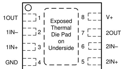
Connect thermal pad directly to GND pin.
