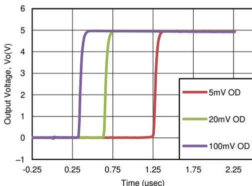
**Figure 4-2. Response Time for Various Overdrives (Positive Transition)**
