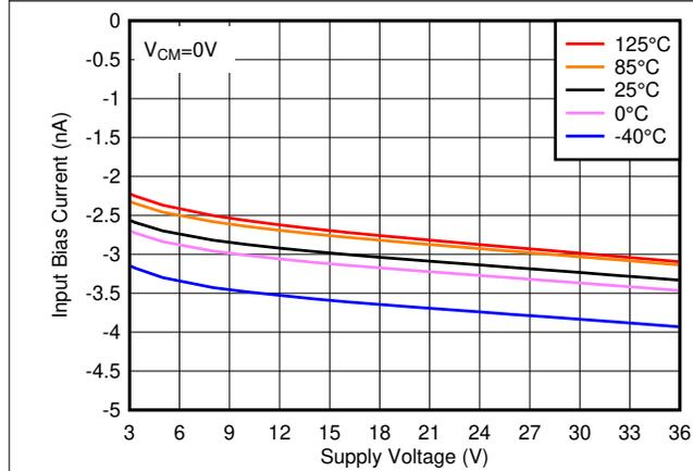
Figure 2-15. Input Bias Current vs. Supply Voltage
