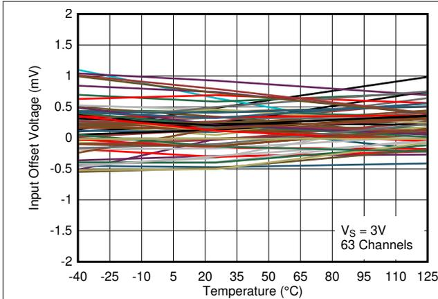
Figure 2-7. Input Offset Voltage vs. Temperature at 3V
