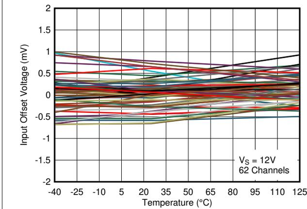
Figure 2-9. Input Offset Voltage vs. Temperature at 12V
