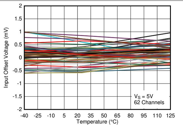
Figure 2-8. Input Offset Voltage vs. Temperature at 5V
