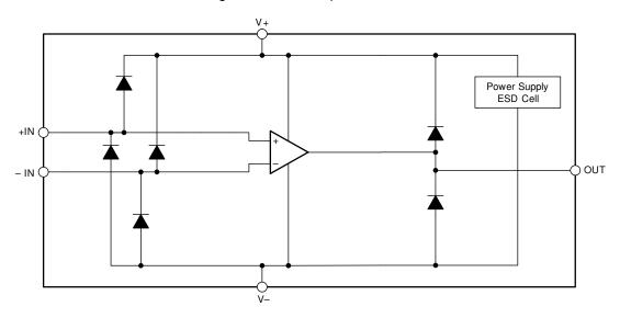
Figure 7-1. Equivalent Internal ESD Circuitry
