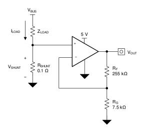
Figure 8-1. LM290xLV Device in a Low-Side, Current-Sensing Application
