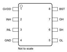
Figure 5-1. D Package, 8-Pin SOIC (Top View)
