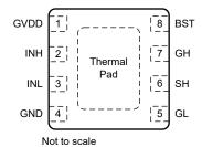
Figure 5-2. DSG Package, 8-Pin WSON (Top View)
