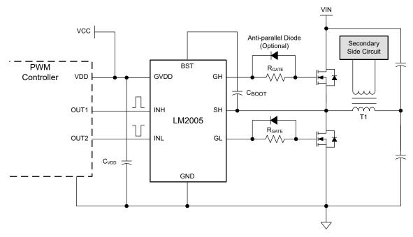
Figure 8-1. LM2005 Driving MOSFETs in a Half-Bridge Converter
