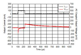
$V_{IN}$  = 5V,  $V_{OUT}$  = 3.3V, ramp rate = 0.4A/ $\mu$ s
