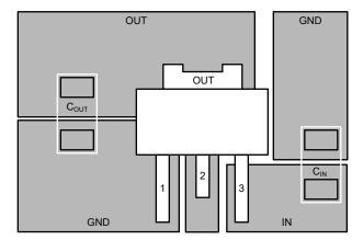
Figure 7-10. Layout Example for KVU (TO-252) Package
