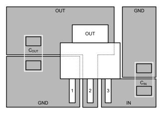
Figure 7-9. Layout Example for DCY (SOT-223) Package
