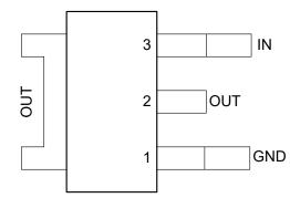
Figure 4-2. KVU Package, 3-Pin TO-252 (Top View)
