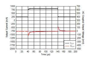
$V_{IN}$  = 5V,  $V_{OUT}$  = 3.3V, ramp rate = 0.8A/ $\mu$ s
