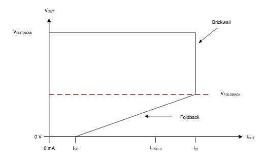
Figure 6-1. Foldback Current Limit
