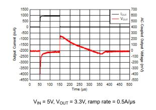
Figure 7-5. I<sub>OUT</sub> Transient From 1mA to 1A
