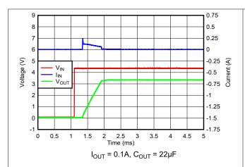
Figure 7-3. Start-up and Inrush Current With 22 $\mu$ F at C<sub>OUT</sub>
